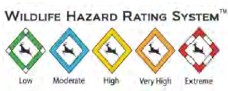
Figure D-51. Variations of deer-vehicle collision warning signs with flashing border intended to alert motorists during peak potential crash periods. Color and flash pattern can be changed as needed. From Sielecki (2017b).
