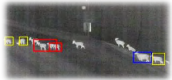
Figure D-54. The British Columbia Ministry of Transportation and Infrastructure used thermal, video, and radar animal detection systems to identify animals of a minimal size and then set off the driver warning systems. Figure Credit: L. Sielecki and British Columbia Ministry of Transportation and Infrastructure.
