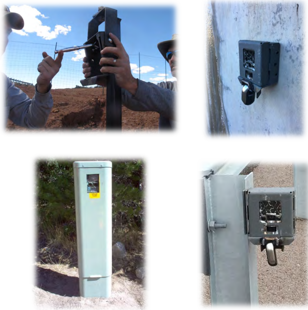
Figure E-10. Camera mounting options: top left - on steel posts mounted in concrete; top right - on concrete wing walls of culvert; lower right - on posts of guard rails; and lower left – in a utility box, Photo Credits: top left – P. Cramer, top right J. Gagnon, lower right J. Gagnon, Lower left, P. Cramer.
