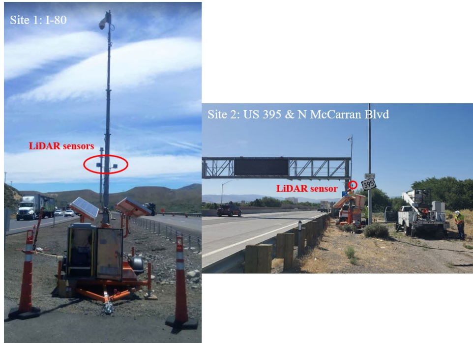
Figure 4-4 ITS trailer equipped with two LiDAR sensors
