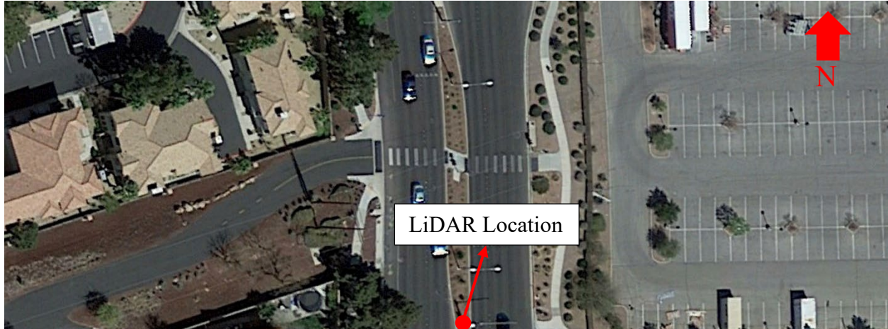
Figure 11-3 Study Mid-Block Crosswalk and LiDAR Location
