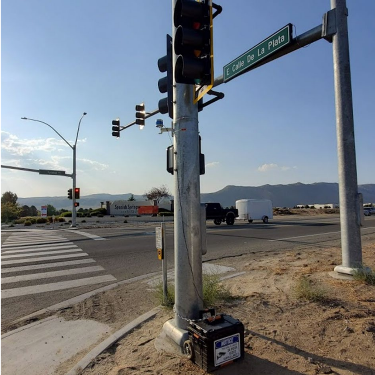
Figure 8-1. Deployed portable LiDAR sensing equipment at the intersection
