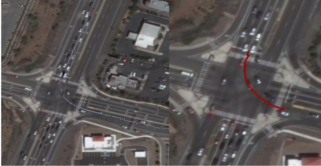
Figure 7-11 Same Vehicle trajectories captured by LiDAR (left) and computer vision (right)
