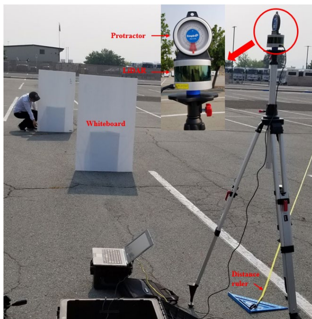
Figure 3-7. Installation position test in a parking lot
