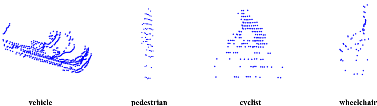
Figure 6-7. Examples of different road user clusters collected by 32-laser roadside LiDAR sensor
