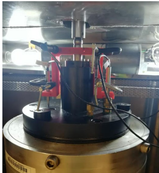
Figure 4.24. LVDTs connected outside the chamber.
