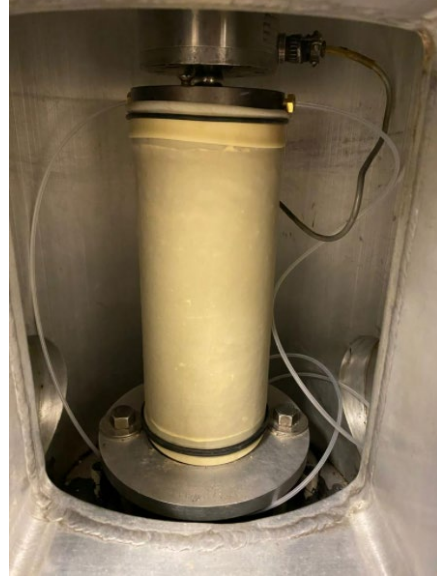
Figure 4.22. Sealed sample in triaxial chamber.
