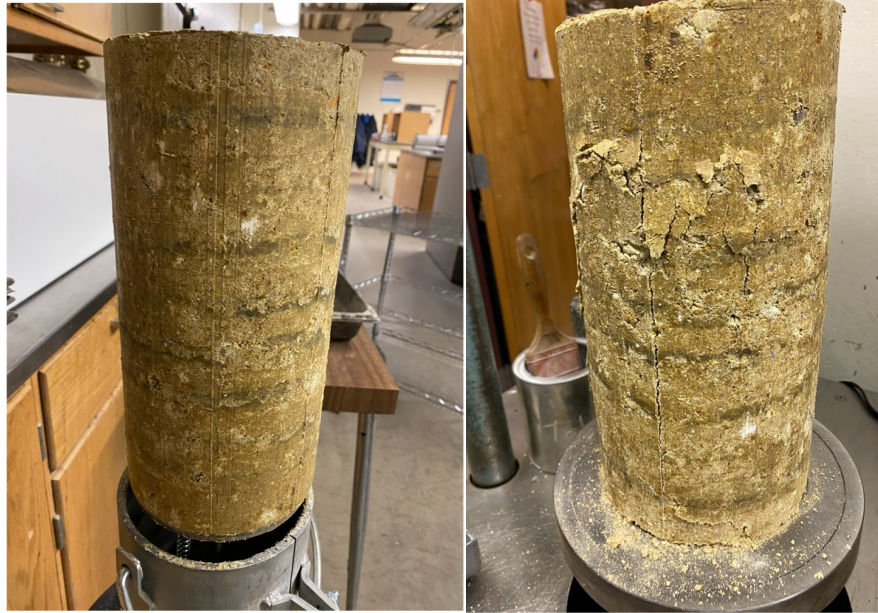
Figure 4.12. Extruded UCS sample. Figure 4.13. UCS sample after testing.
