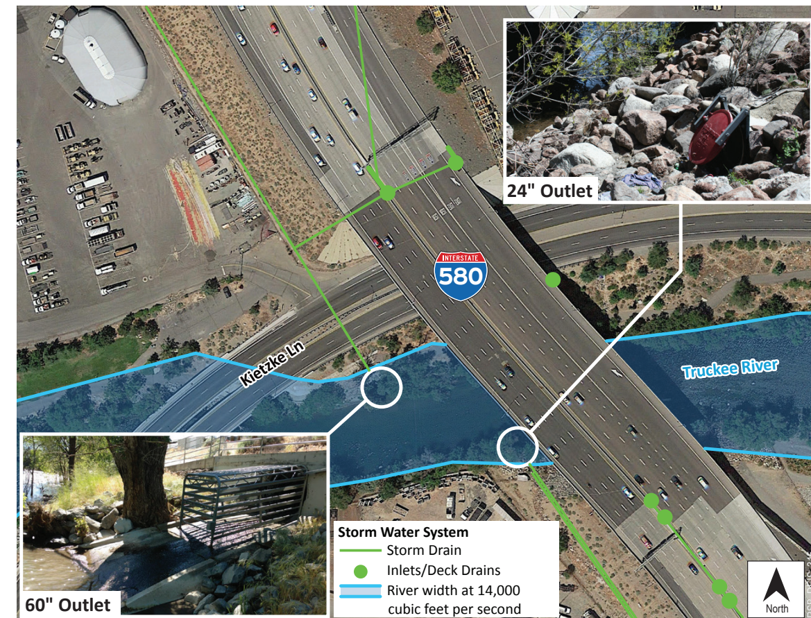
Figure 3.8-2. I-580 Stormwater Discharge Points into the Truckee River
