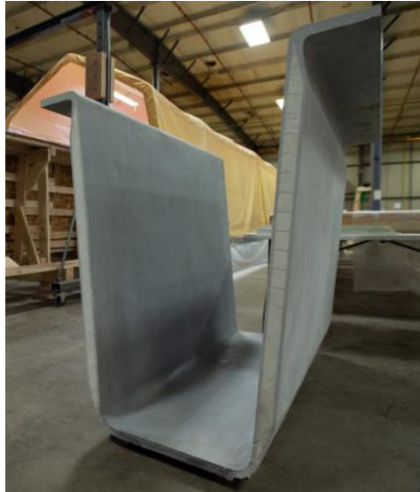
Figure 17: A section of a CT Girder made by AIT. Foam inserts can be seen in the vertical walls of the girder to help reduce the weight.
