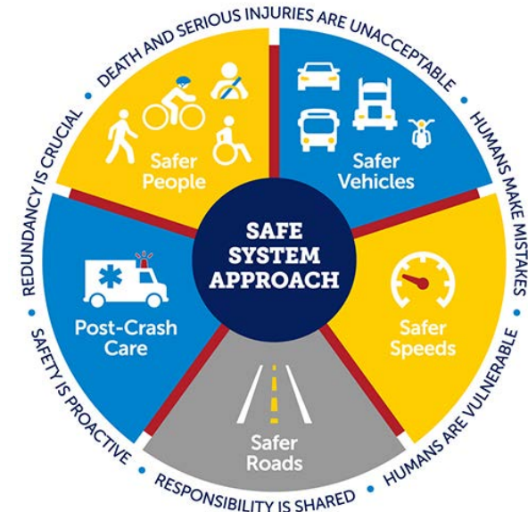
Figure 13: Safe System Approach (source: U.S. DOT)
