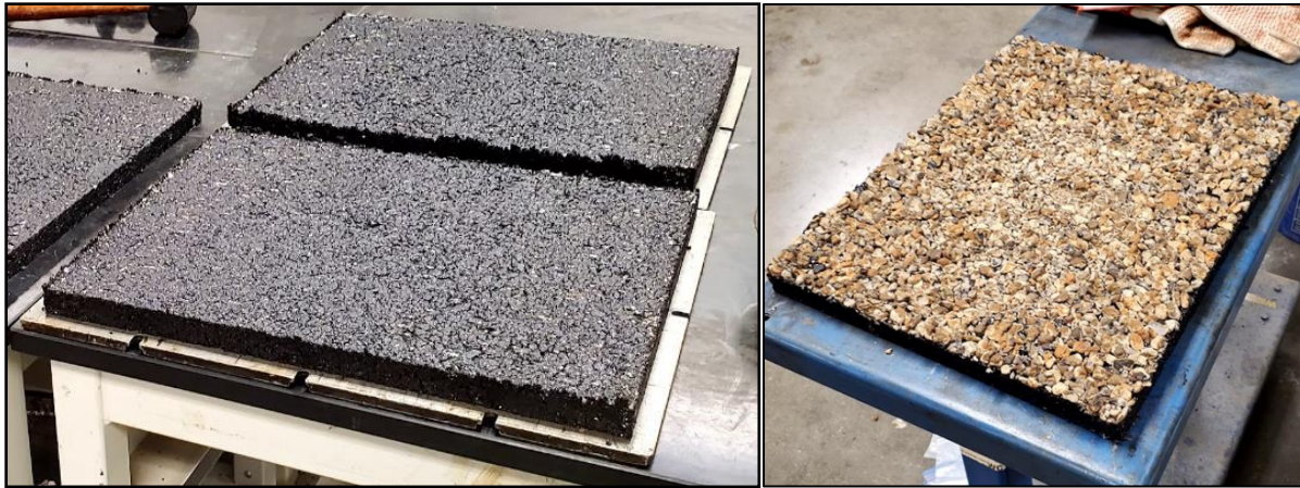
Figure 2: HMA slab with ST preparation.
