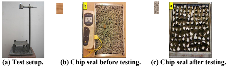
Figure 3. Vialit test for raveling of chip seals.
