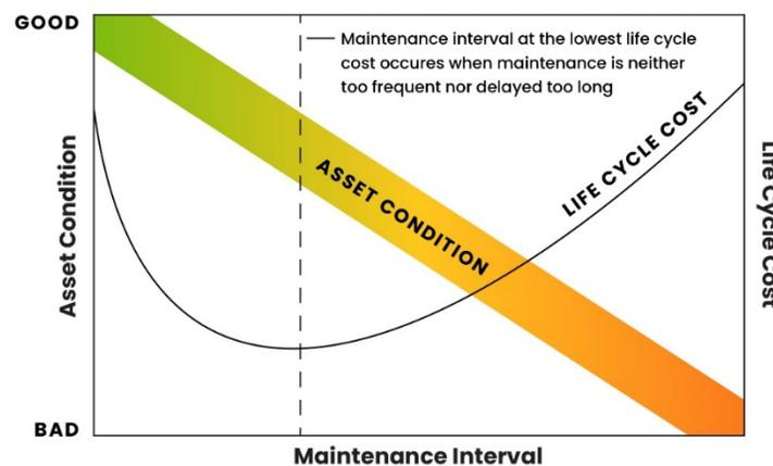
Figure 4-2. Illustration of the life cycle cost analysis concept.
