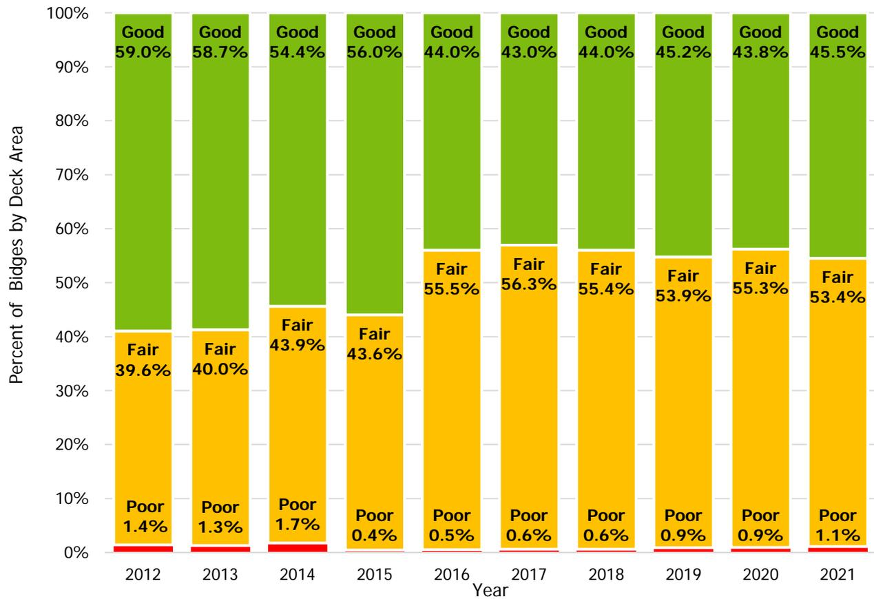
Figure 3-8. Bridge performance trends for NHS and state-owned NBIS bridges.<sup>4</sup>
