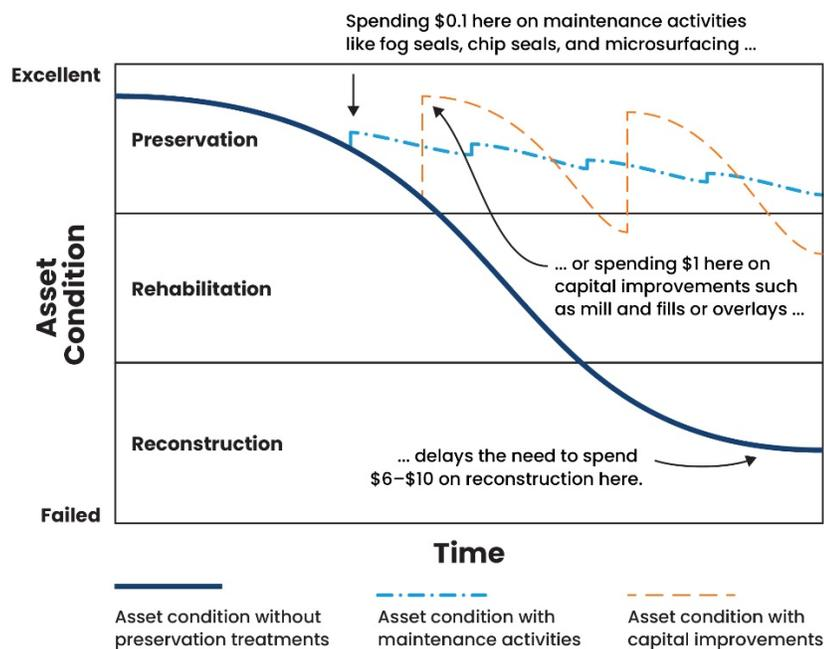
Figure 4-3. Conceptual model of asset deterioration and treatment strategies.
