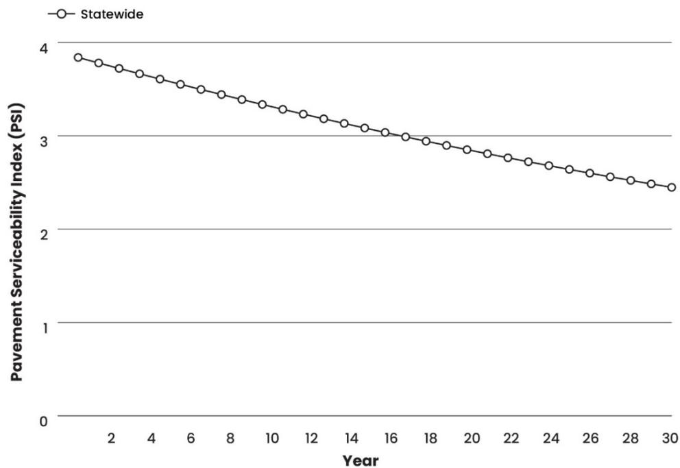
Figure 4-5. Concrete pavement condition deterioration model used by NDOT.
