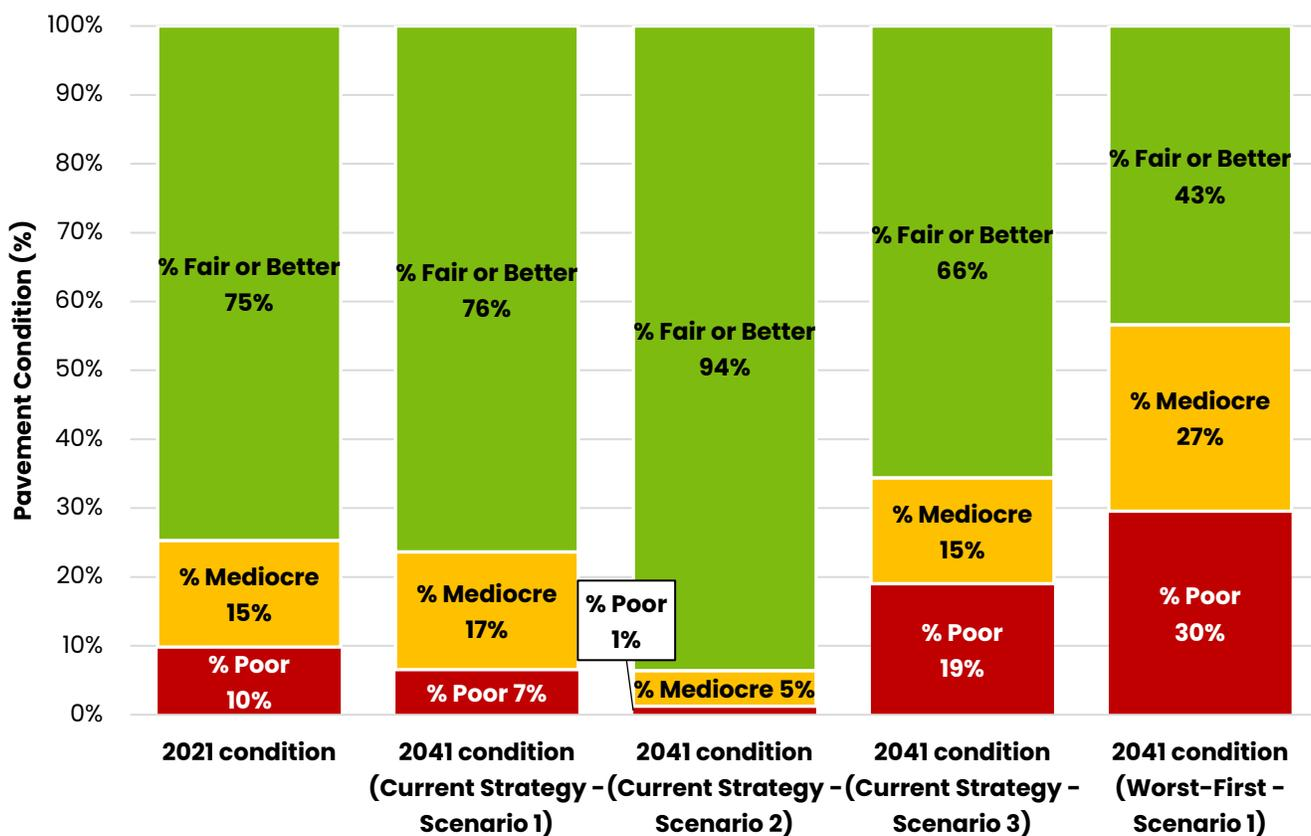
Figure 4-9. Initial and projected statewide pavement condition for each LCP analysis run.
