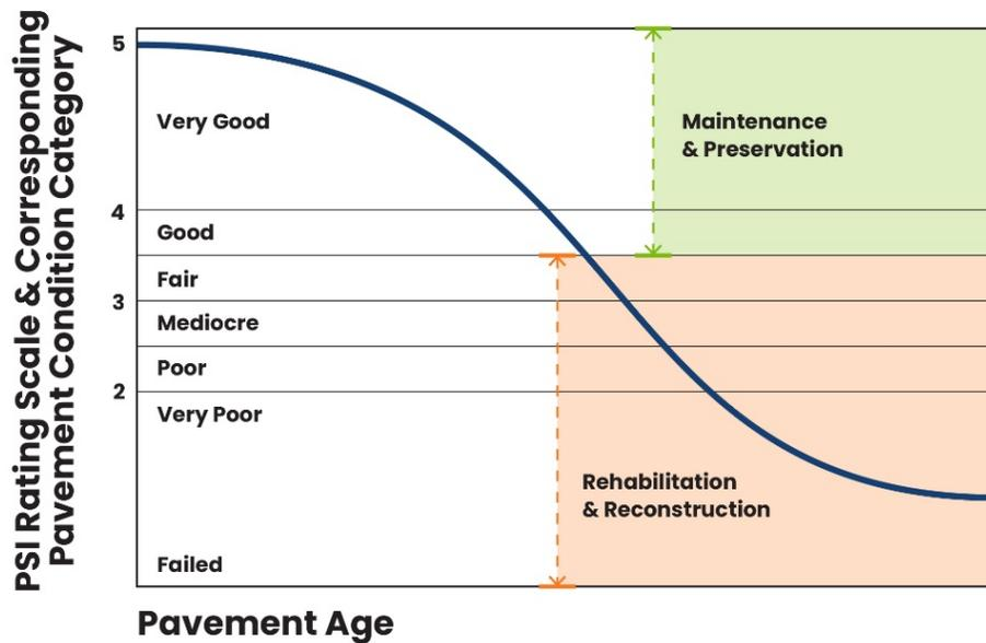
Figure 4-7. Illustration of a typical pavement deterioration curve and suitable repair strategies based on the PSI rating.
