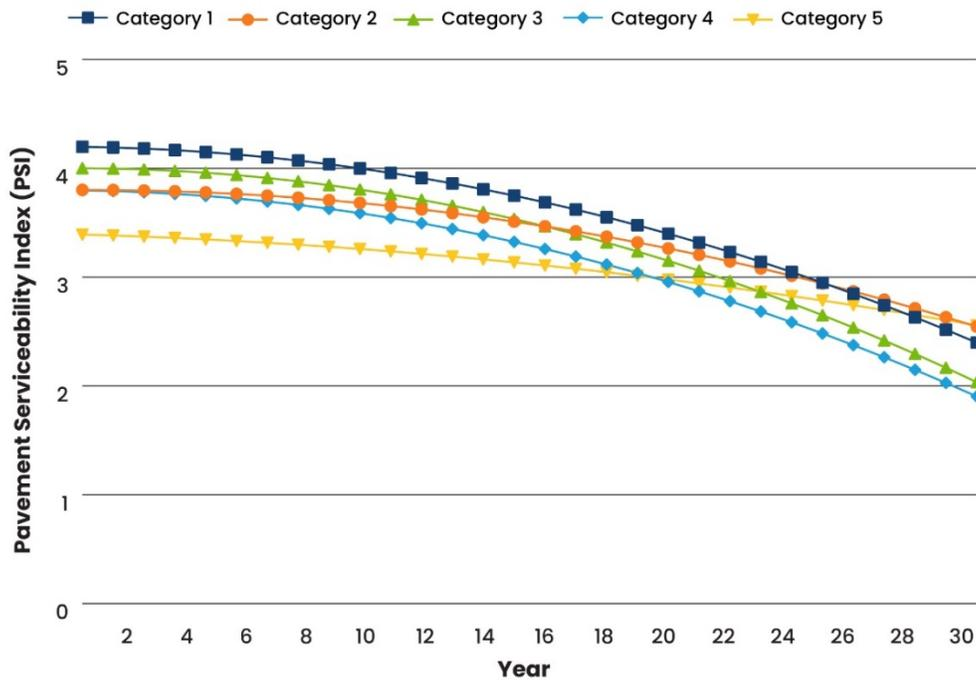
Figure 4-4. Asphalt pavement condition deterioration models used by NDOT.
