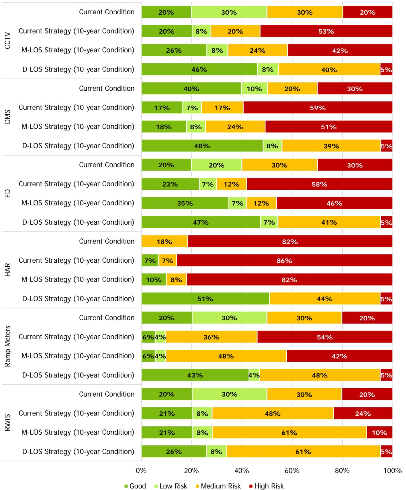
Figure 4-14. Comparison of current and projected 10-year ITS asset conditions.
