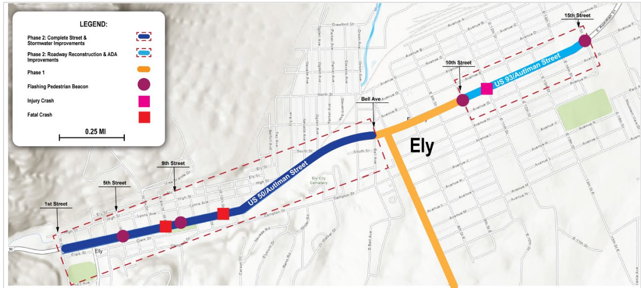
Figure 6. Flashing Pedestrian Beacons Installed Near Prior Crash Locations
