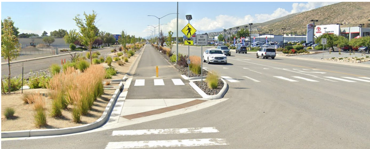
A barrier-separated trail along Business Route 395 in Carson City. This is an example of using plantings, lighting, a Rectangular Rapid Flashing Beacon at a crossing, and physical separation to increase walking and biking. Source: Google Maps 2024
