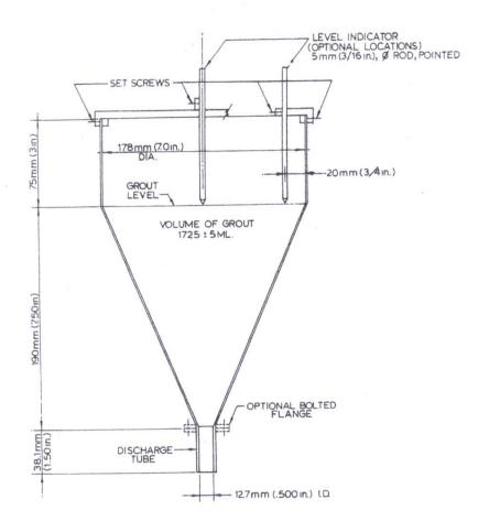
Figure 1 - Cross Section of Flow Cone
