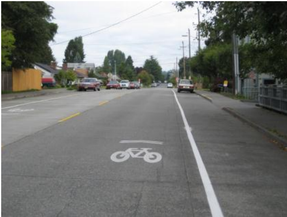
Figure 6 – Marked Shared Lane Facility
