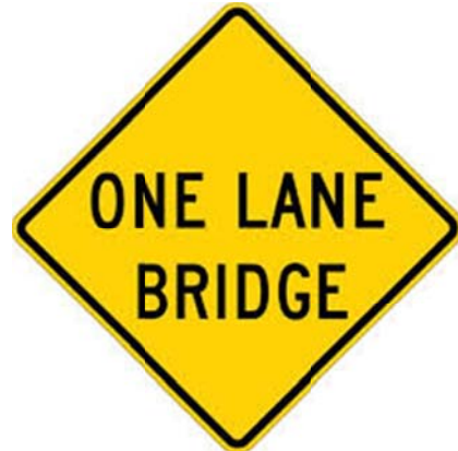
W5-3 – One Lane Bridge Sign
