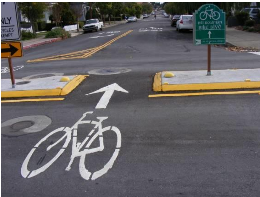
Figure 7 – Bicycle Boulevard Facility
