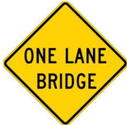
W5-3 – One Lane Bridge Sign
