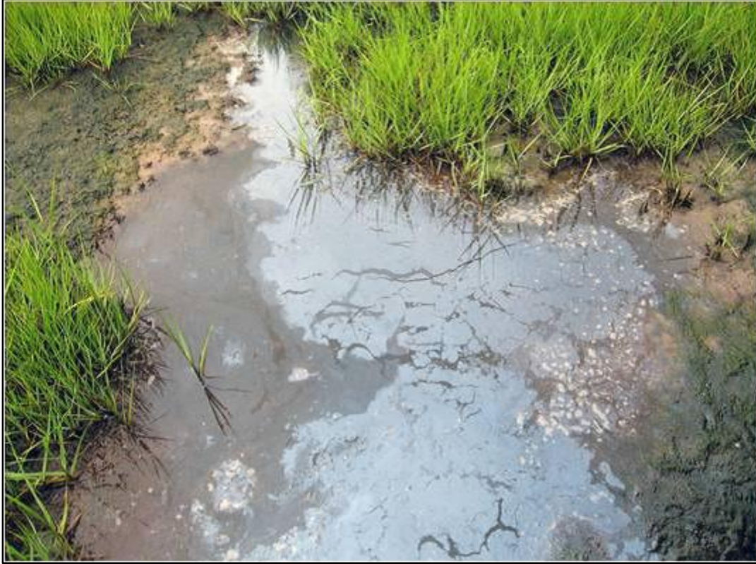
Figure 1-25. This sheen is caused by the natural decay of plant matter and is not associated with an illicit discharge. Note the dullness of the sheen and how it tends to break apart rather than flow. (Photo from the Center for Watershed Protection)
