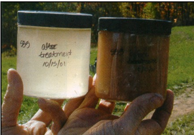
Figure 1-19. A lightly turbid water (left) and highly turbid water (right). (Photo from the City of Reno)
