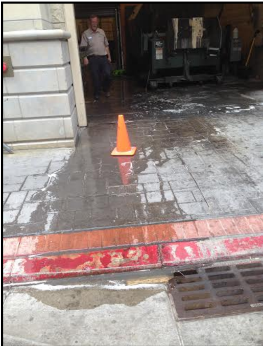
Figure 1-4. In this situation, a garbage pad area is being washed down with no means of protection or attenuation of pollutants from reaching the MS4. This is regarded as an indirect mode of entry and transient in that it only periodically discharges to the storm system. If this is their routine maintenance practice, it could be considered an “ intermittent ” discharge. (Photo from T. Svetich)
