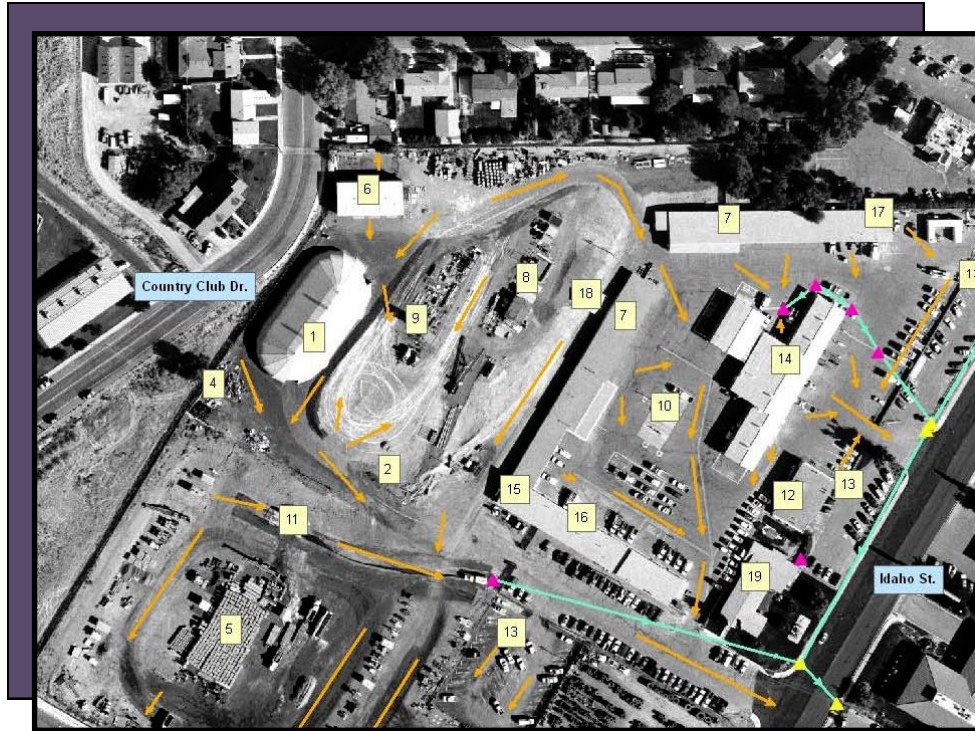
Map of Elko NDOT maintenance facility with depiction of stormwater flow directions, catch basins, and storm drain piping.
