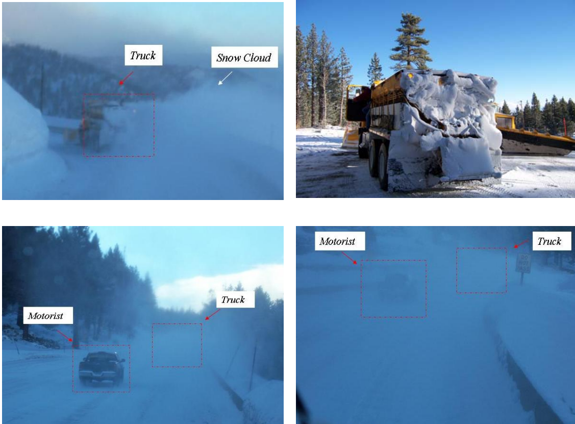
Figure 1.2 Covered Lights and Visibility Impairment behind the Truck (Mount Rose Highway, Washoe County, NV, March 2006)
