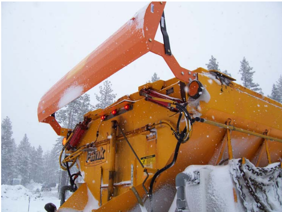
Figure E 3. Alternative Installations of Airfoil
