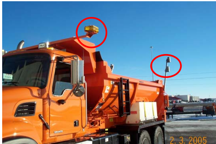
Figure A.1 North Dakota Warning Lights Positioned Away from the Dump Body
