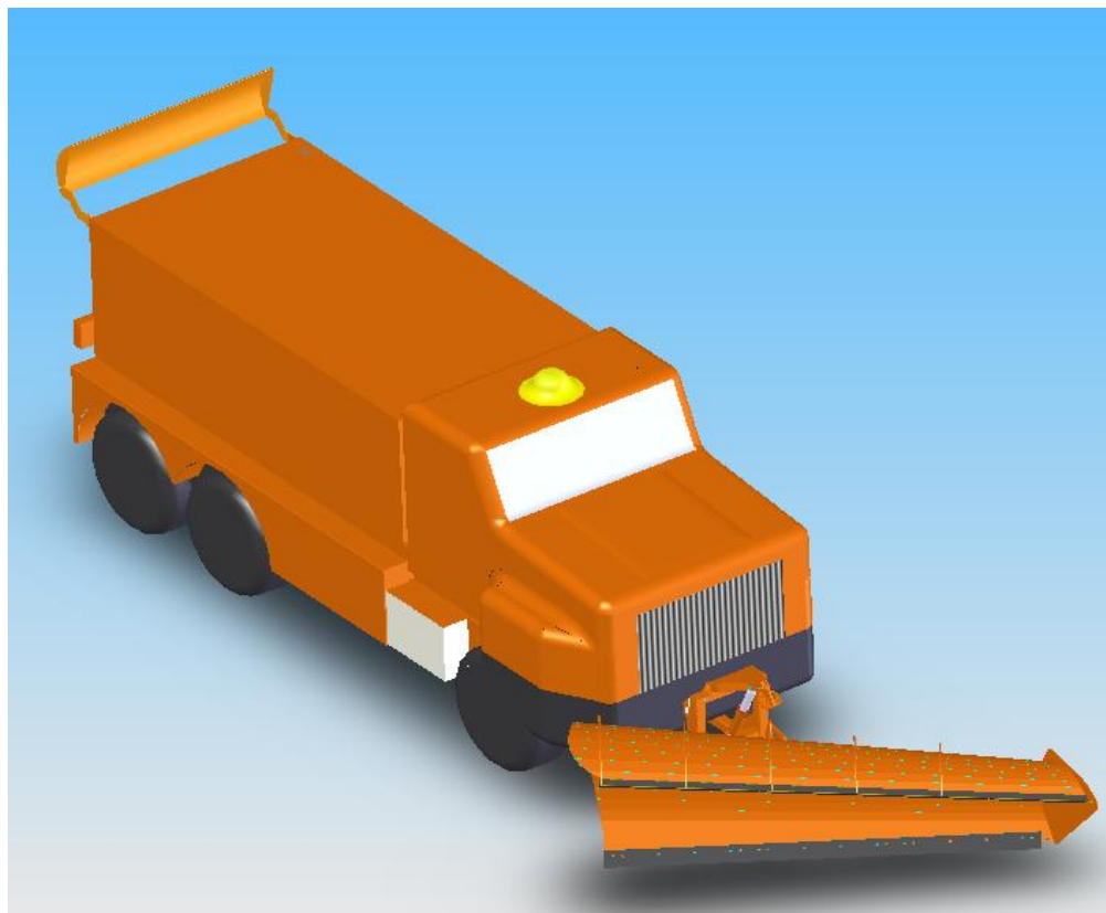
Figure B.1 Three Dimensional Model of Class-15 Truck and Henke-4806 One-way Plow with Monroe Airfoil Mounted on the Sander
