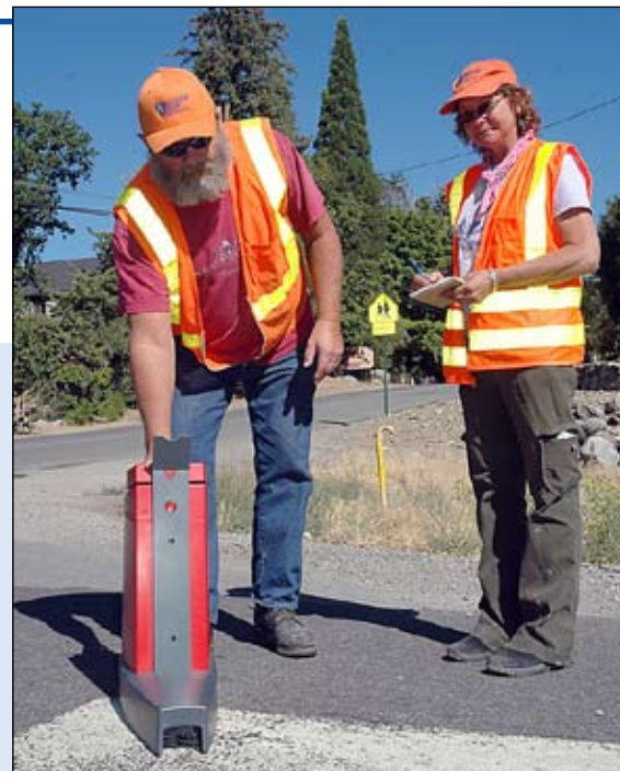
With the help of crew 241's Susan Linn (pictured on right), Crew Supervisor Jim Boston demonstrates how reflectometers are used to measure the reflective properties of school zone crosswalks.
