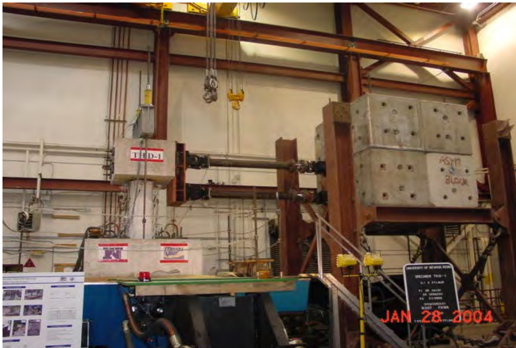
Figure 3-8 Test Setup of Specimen THD-1, THD-3, THD-5
