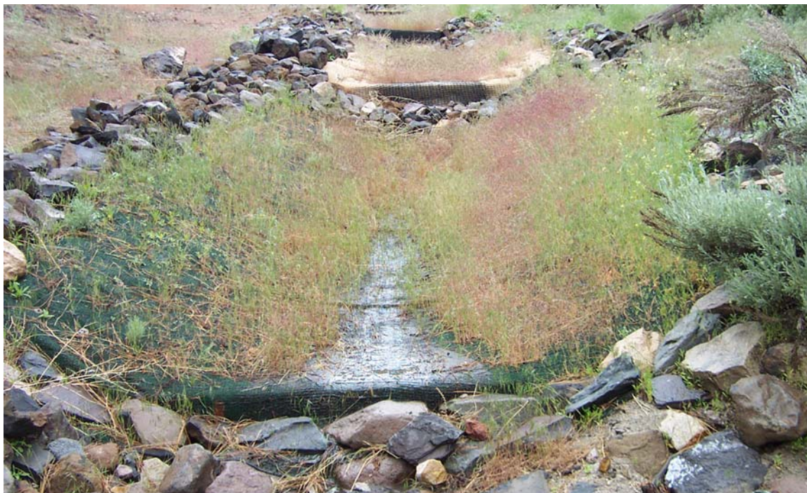
Figure 4.36 Field plot lined with SI Geosolutions Landlok 450 looking upstream (June 2005).
