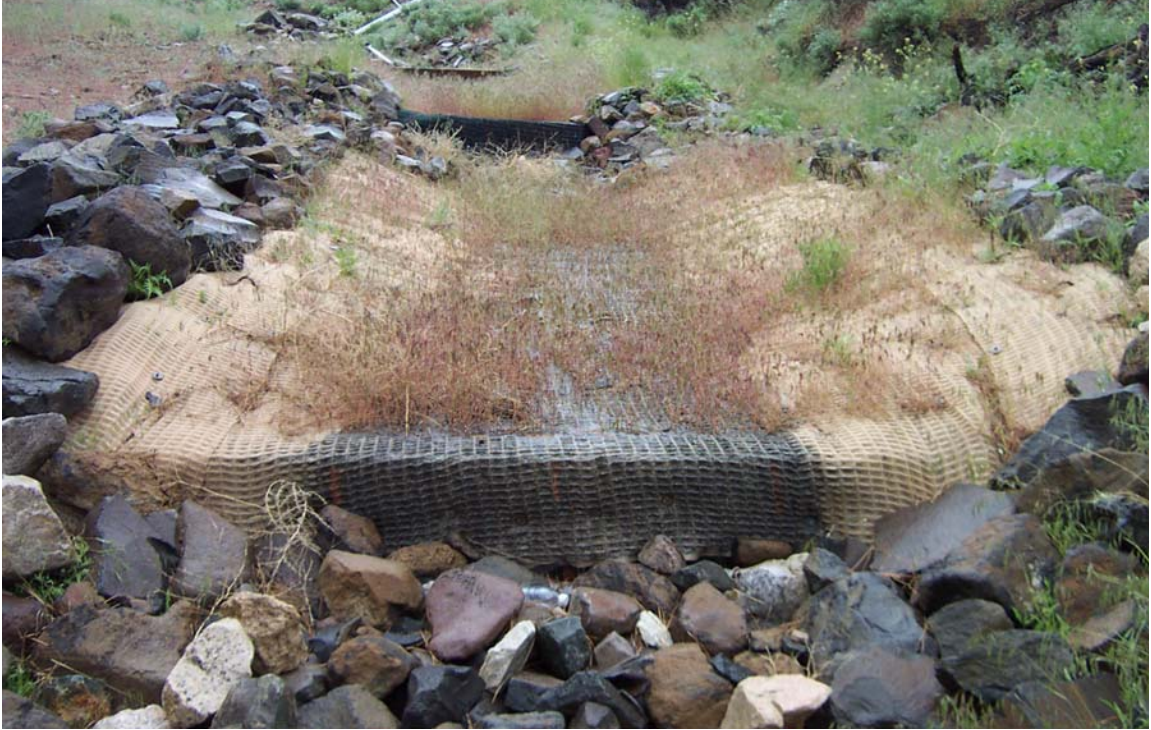
Figure 4.34 Field plot lined with SI Geosolutions Pyramat looking upstream (June 2005).
