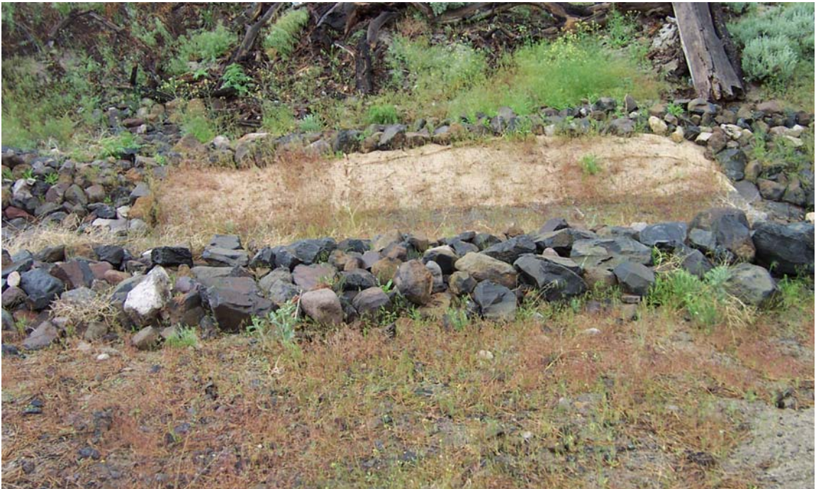
Figure 4.34 Field plot lined with SI Geosolutions Pyramat looking upstream (June 2005).
