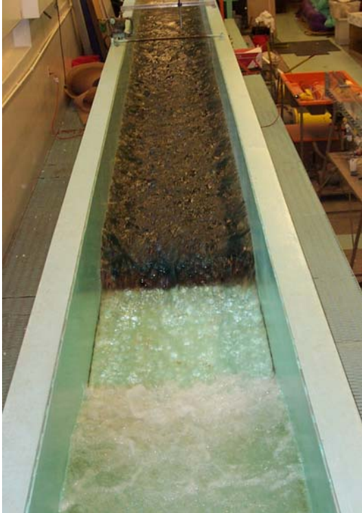
d) Flow Test Showing Hydraulic Jump
