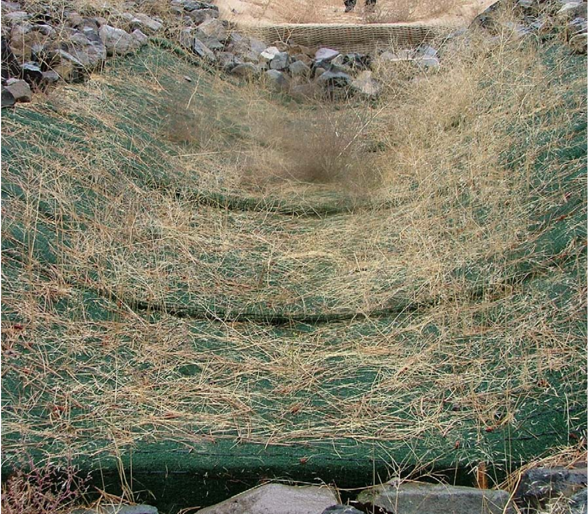
Figure 4.26 Field plot with SI Geosolutions Landlok 450 looking upstream (November 2004).
