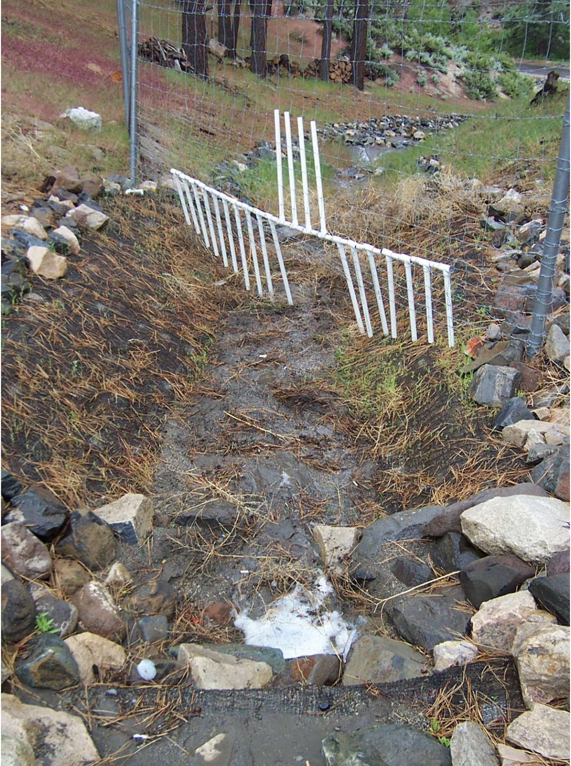
Figure 4.39 Field plot lined with North American Green SC250 looking downstream (June 2005).
