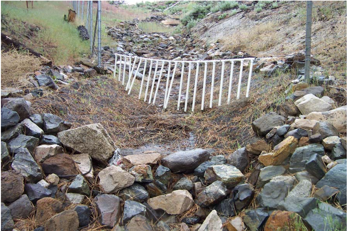
Figure 4.38 Field plot lined with North American Green SC250 looking upstream (June 2005).
