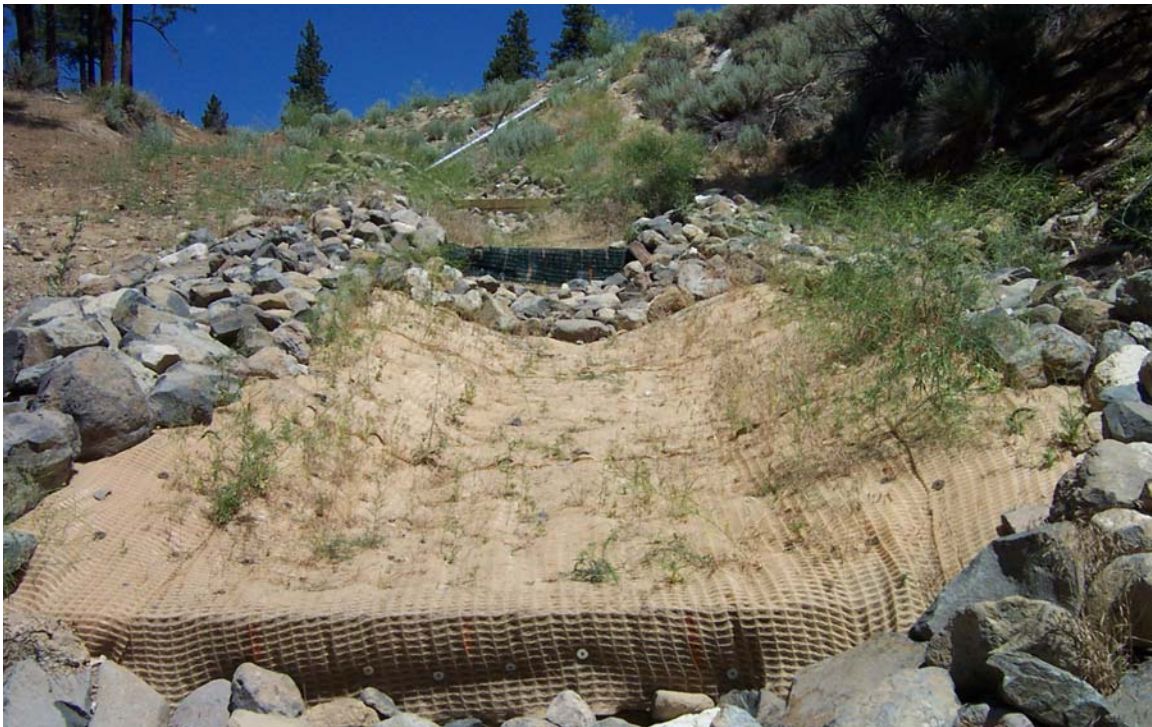
Figure 4.21 Field plot with SI Geosolutions Pyramat looking upstream (July 2004).
