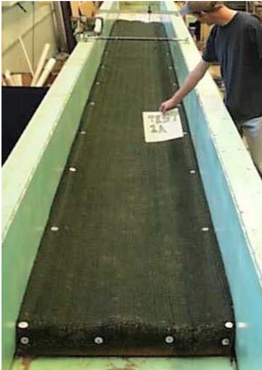
c) TRM Installed, Ready for Test
