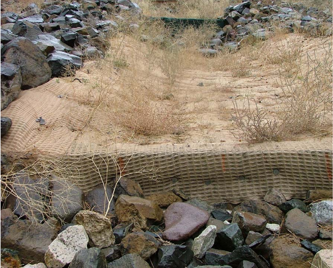
Figure 4.25 Field plot with SI Geosolutions Pyramat looking upstream (November 2004).
