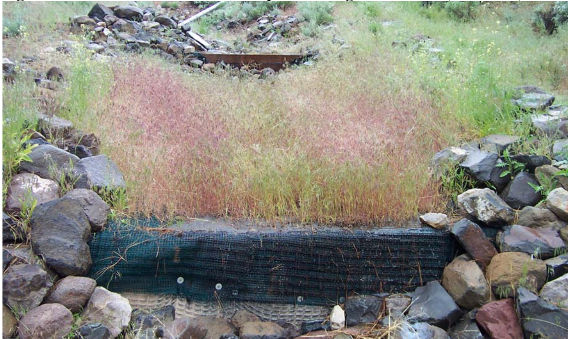
Figure 4.32 Field plot lined with North American Green P550 looking upstream (June 2005).
