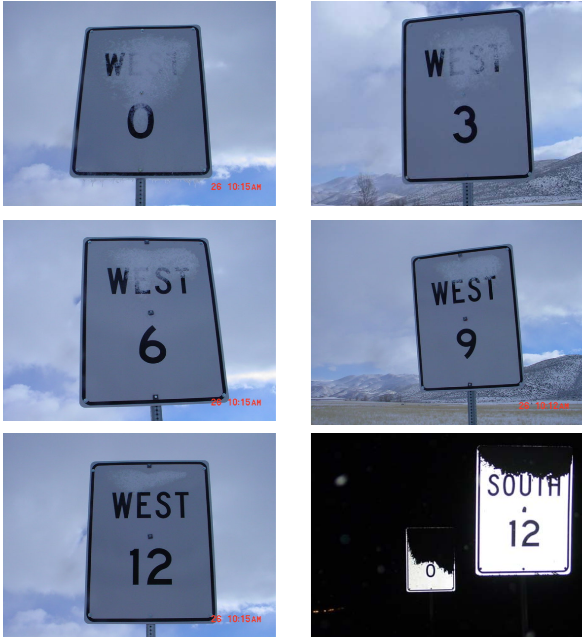
Figure 3-3. Illustrates the Snow Accretion as Function of Sign Tilt (Storm date 2-26-2004)
