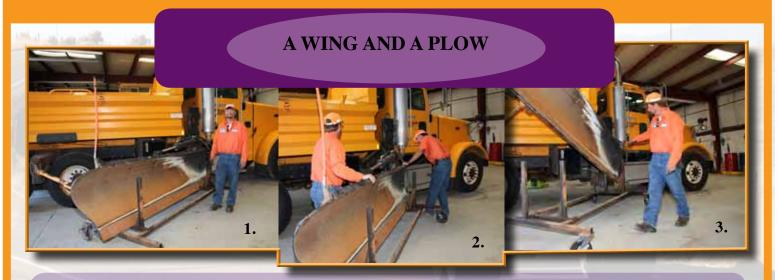
Pictured at left, Bill Hylton stands beside the cart he designed which makes it as easy as 1,2,3 to install snow plow side wing blades.
