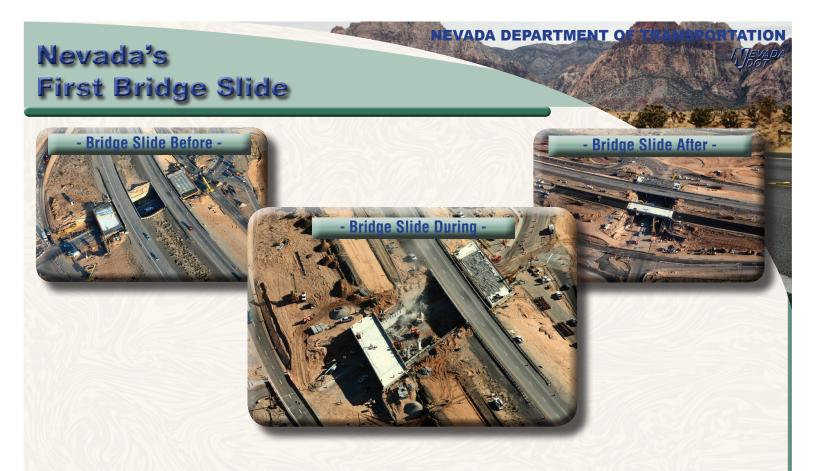
Two Interstate 15 bridges were demolished and replacement bridges slid in place as part of the first bridge slide in state history, and cornerstone of an NDOT project to improve the I-15 interchange 120 in Mesquite.
