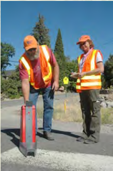
To help protect the safety of school children and motorists, NDOT maintenance professionals use reflectometers to measure the reflectivity of school zone crosswalks.
