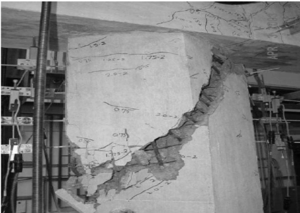
Figure 6-7 Shear Failure of the South Column during Run 23
