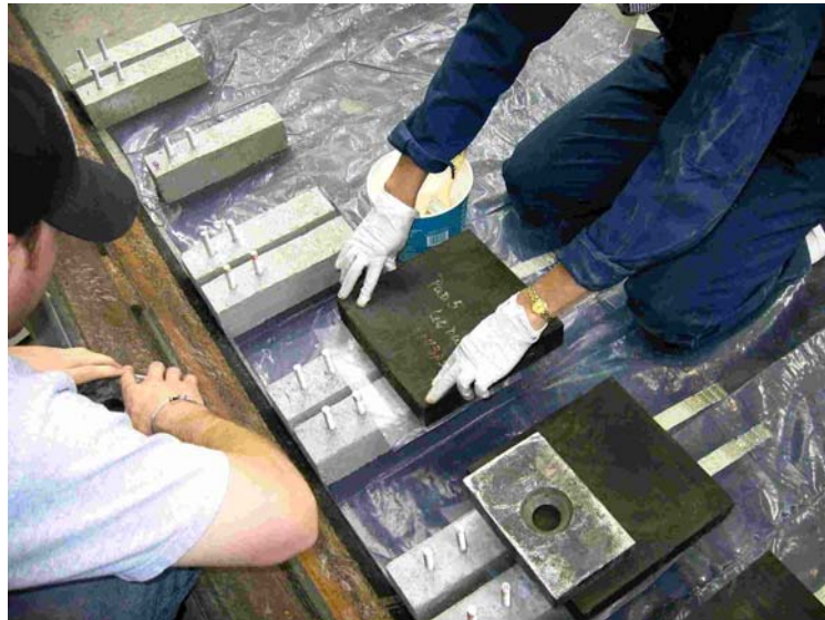
(b) Covering Bonded Strips with Polyurethane and Weights.
