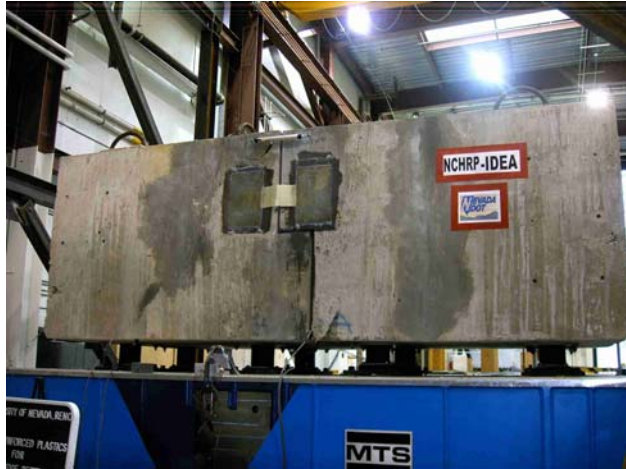
Figure 5-1: GFRP restrainer shake table tests
