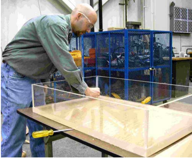
(a) Arranging Acrylite Sheets into Vacuum Box
