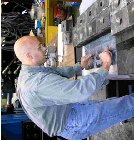
(b) Pressing excess epoxy from fabric
