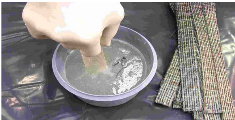
Figure 2-9: Dipping Ends of Fabric Strips into Resin
