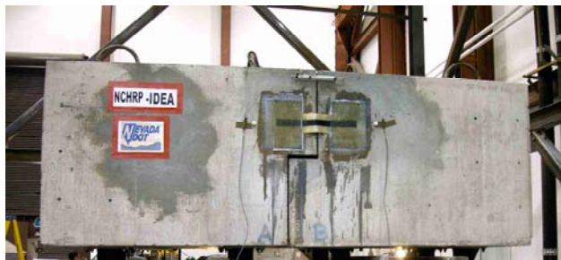
Figure 5-3: CGFRP restrainer shake table tests
