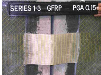
(a) PGA of 0.15g, north-side restrainer
