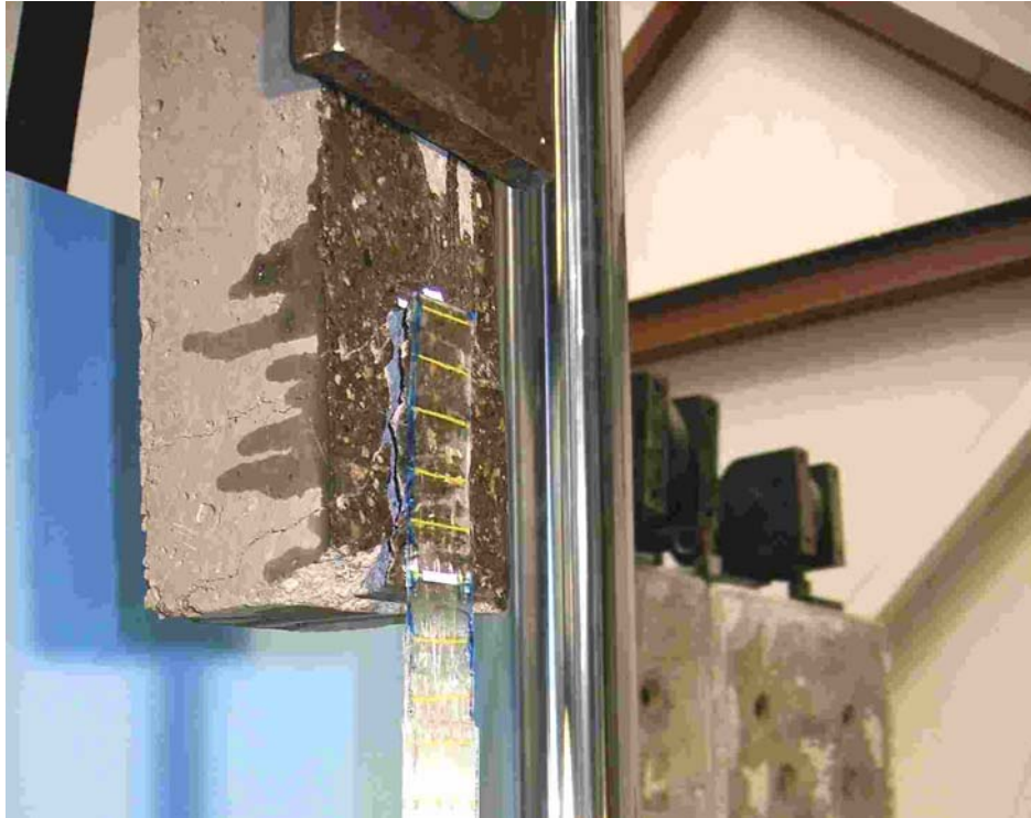
Figure 2-151: Bond Failure during Tensile Tests
