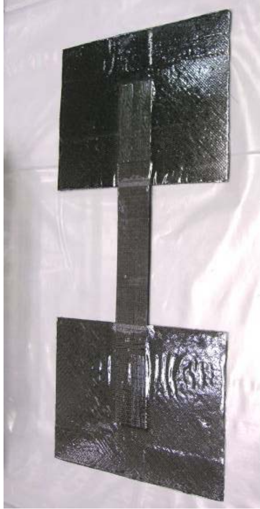
(e) Completed CFRP restrainer
