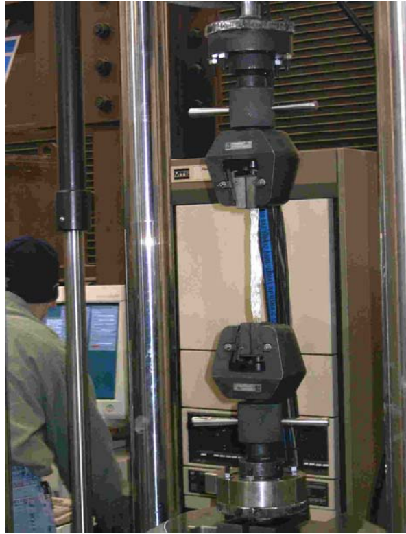
Figure 2-6: Material Tensile Tests Using MTS Load Frame
