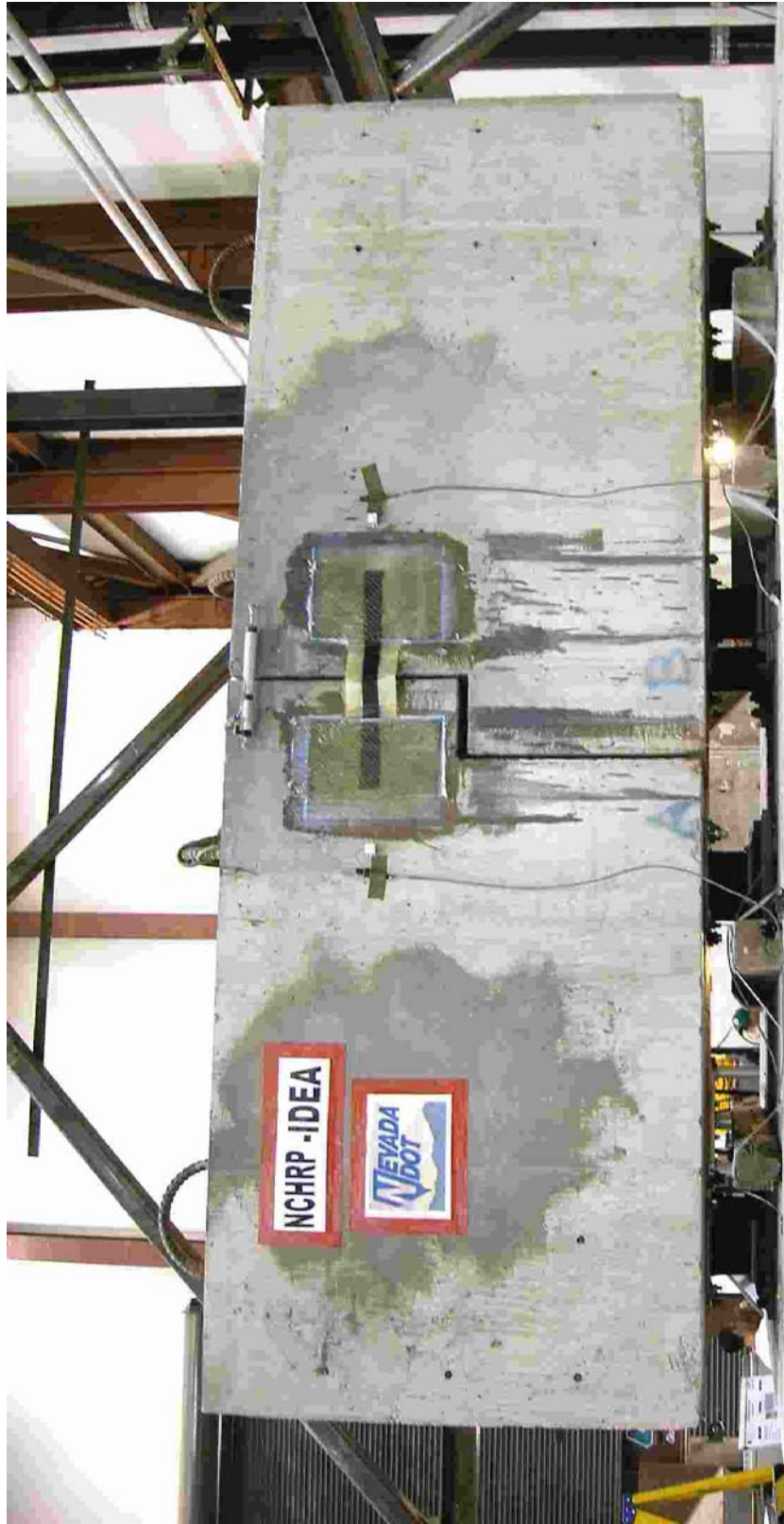
Figure 4-1: Test set-up for FRP bridge restrainer shake table experiments.
