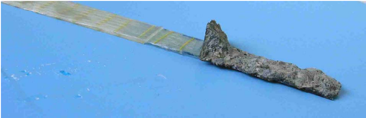
Figure 2-152: Close-up of Bond Failure
