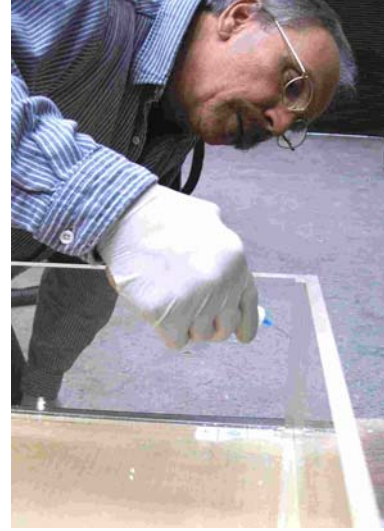
(b) Forming Box with Weld-On
