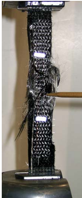
(b) Plain Fabric Strips with Increasing Rate (Left to Right) from Low to High Dynamic Rate
