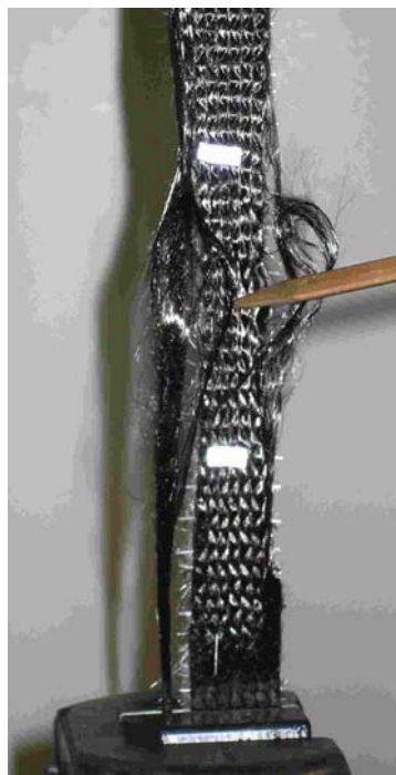
Figure 2-11: Typical Failure Mode of Carbon Fabric Strips
