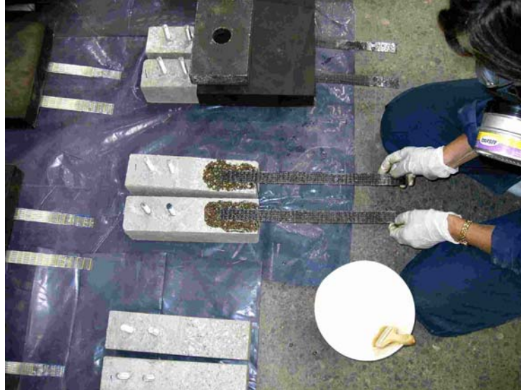
(a) Strips being Epoxied to Concrete Blocks
