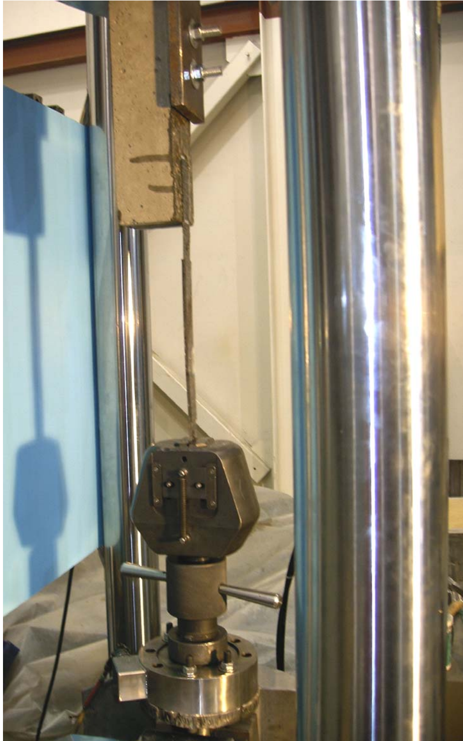
Figure 2-144: FRP/Concrete Bond Tests on MTS Load Frame
