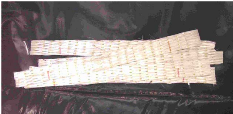
Figure 2-8: Glass Fabric Strips with Ends Marked for Epoxy Application
