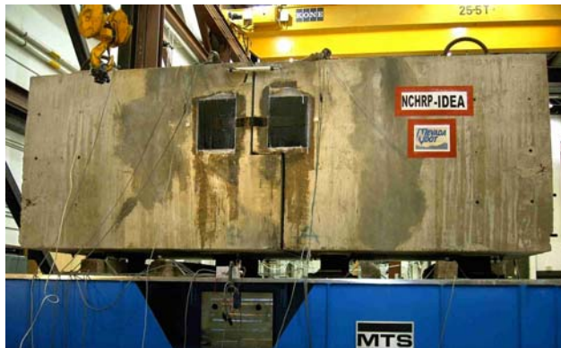
Figure 5-2: CFRP restrainer shake table tests
