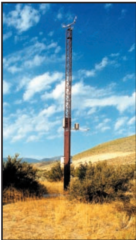
Road Weather Information System technology collects vital information that results in reduced application of sand and salt at Lake Tahoe.
