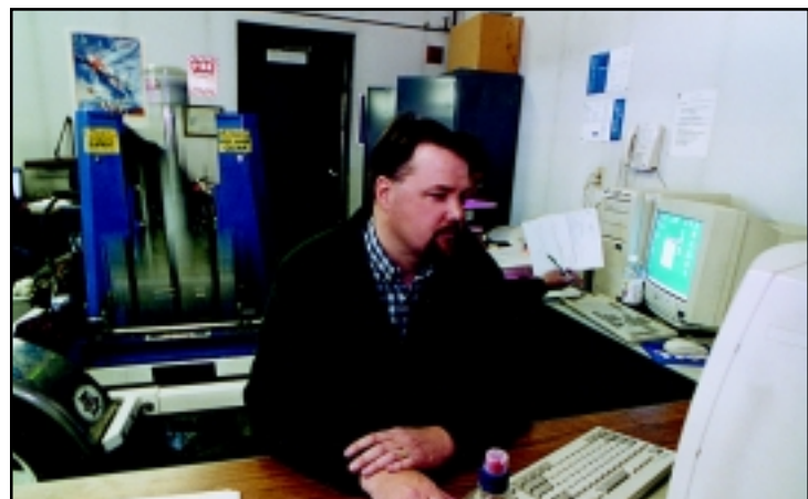
TESTING—Chris Joncas runs the testing lab in Reno, which serves state departments of transportation throughout the west. Here he watches the impact registered on the computer from the falling weight on the deflectometer behind him.
