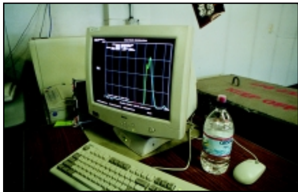
BOUNCE! —The impact of several thousand foot pounds of force hitting a load cell registers plainly on the computer monitoring the deflectometer test.
