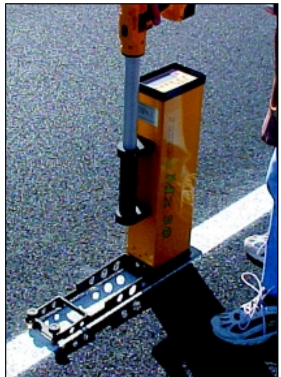
PRECISION LOOK—This machine measures the reflectivity of the pavement marking right after it is applied, and a later test will see how well the material performs over time.
