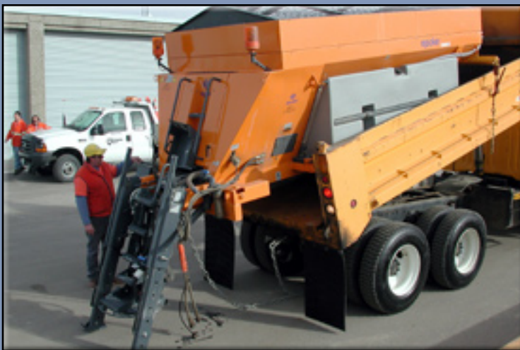
LATEST TECHNOLOGY —Larry Hough guides a new Epoke combination sand/salt spreader onto a snowplow truck bed. The spreader lays down granules or brine in precise, directed amounts. The operator can send material straight behind his machine, or to the side, covering one or two lanes. The accurate delivery system ensures that unnecessary material is not put out on the road, minimizing pollution and waste.
