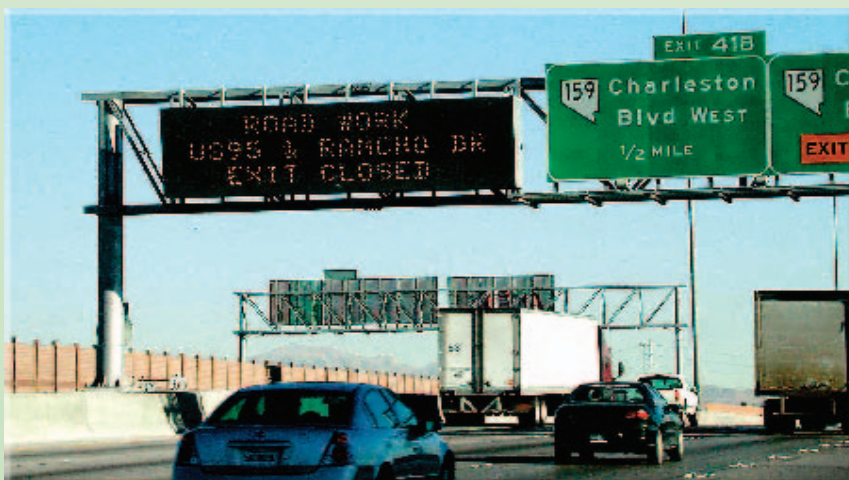
DMS—Dynamic Message Signs in southern Nevada are controlled from the Freeway and Arterial System of Transportation (FAST). With 12 DMS signs in southern Nevada, the public has an early warning system to make a lane change because of an accident ahead or closed off ramp.
