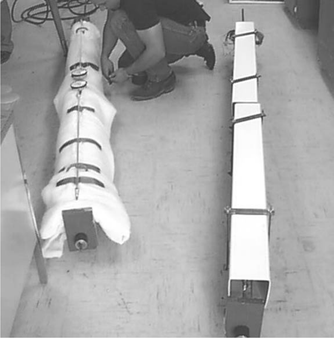
Figure 3.11 – Solid Beams with Mechanical Gage Cover and Batting for Moist Curing Prior to Gage Cover
