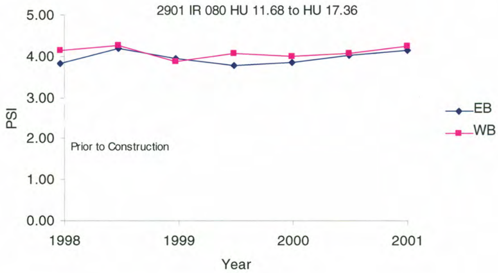
Figure 22. Contract 2901 PSI Performance
