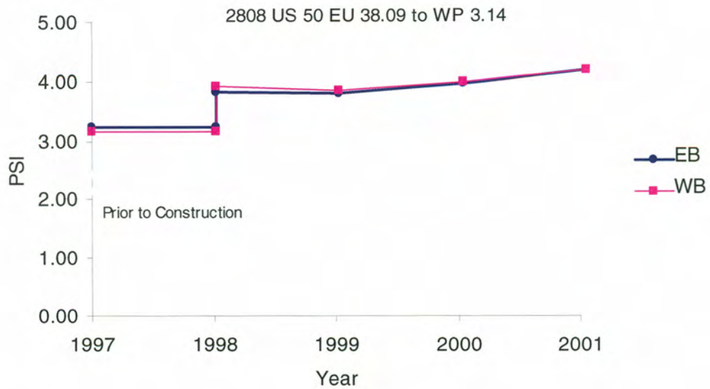
Figure 2. Contract 2808 PSI Performance
