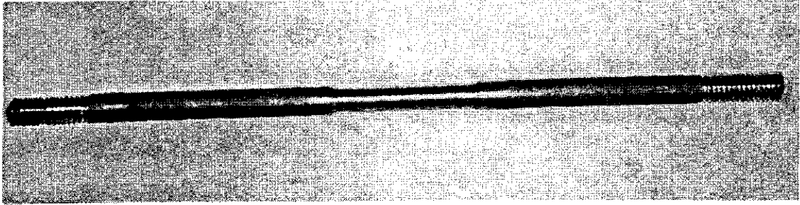
Figure 2-26: Reduced Section and Threads on 0.375-in NiTi Bar
