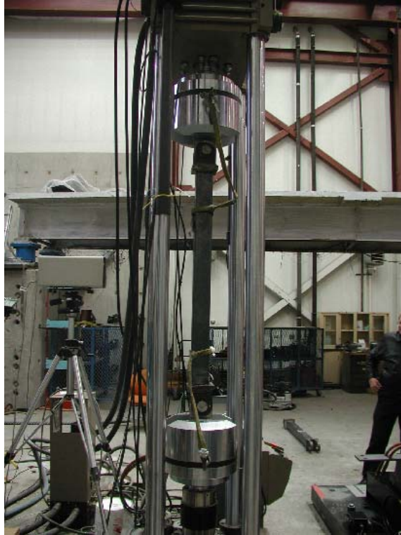
Figure 2-20: Specimen in the Vertical Testing Machine
