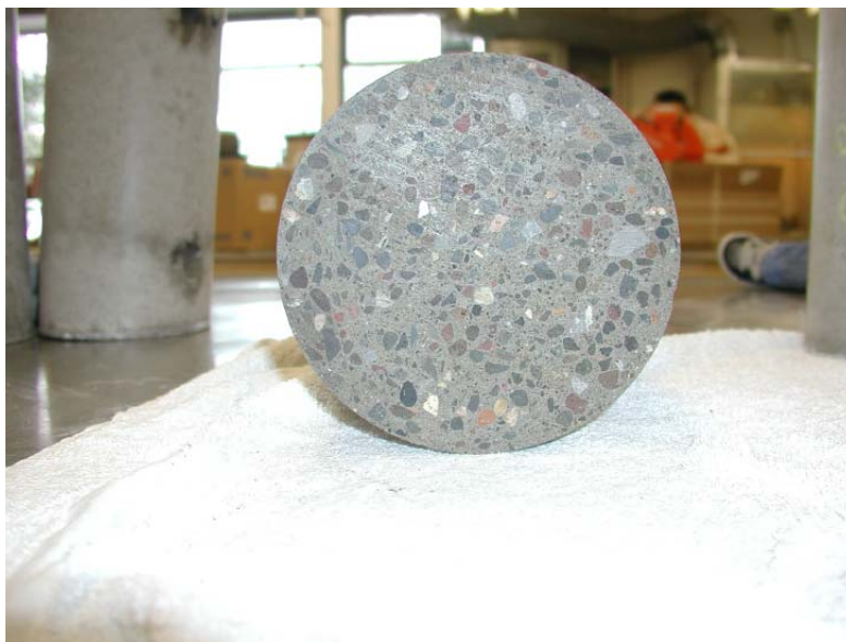
Figure 2-3: Cross-Section of Cut Cylinder from PVC Pipe Specimens
