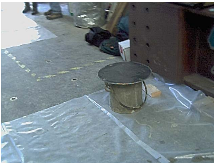
Figure 2-10: Metal Bucket and Cover for Bleed Water Test
