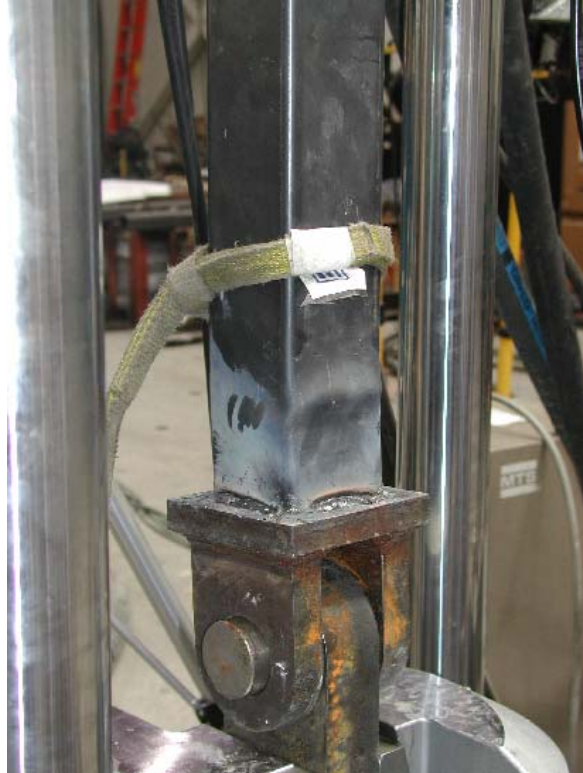
Figure 3-16: First Test Local Buckling at Bottom
