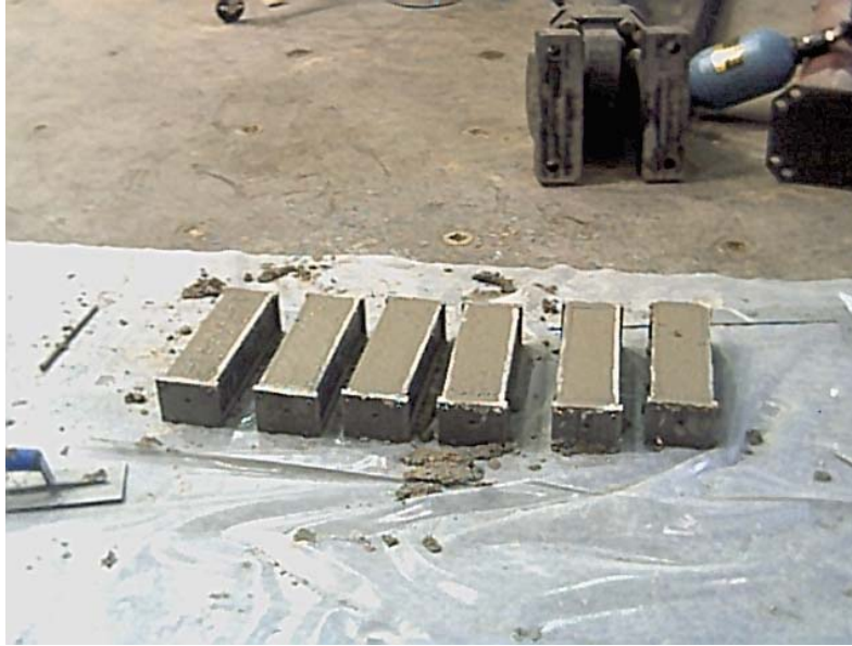
Figure 2-6: 3-in x 3-in x 11.25-in Prism Molds for the Length Change Test
