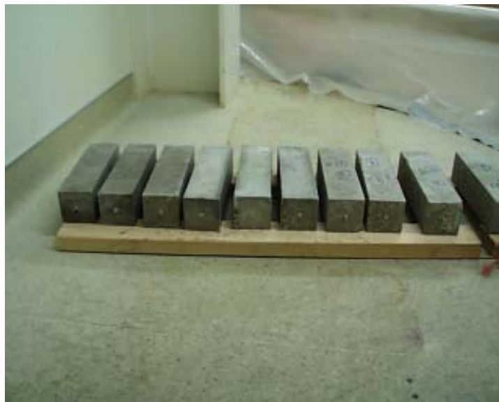
Figure 2-9: Specimens Air Curing
