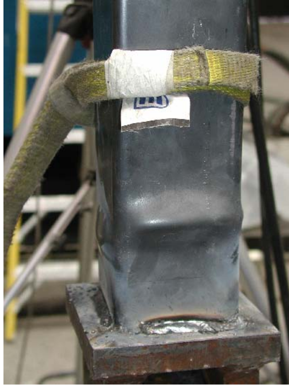
Figure 3-17: First Test Local Buckling Close-Up
