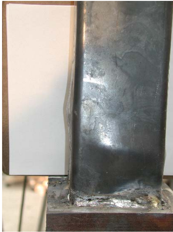
Figure 3-19: Second Test Local Buckling All Four Sides
