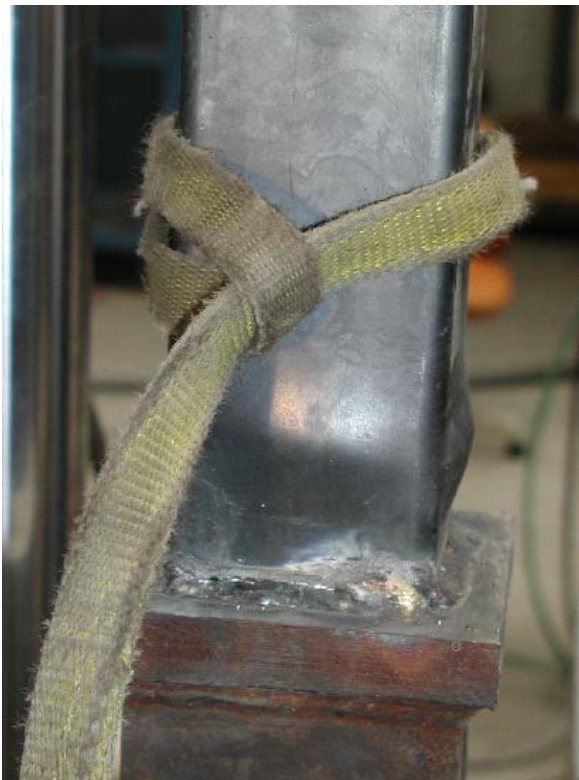
Figure 3-18: Second Test Local Buckling at Bottom
