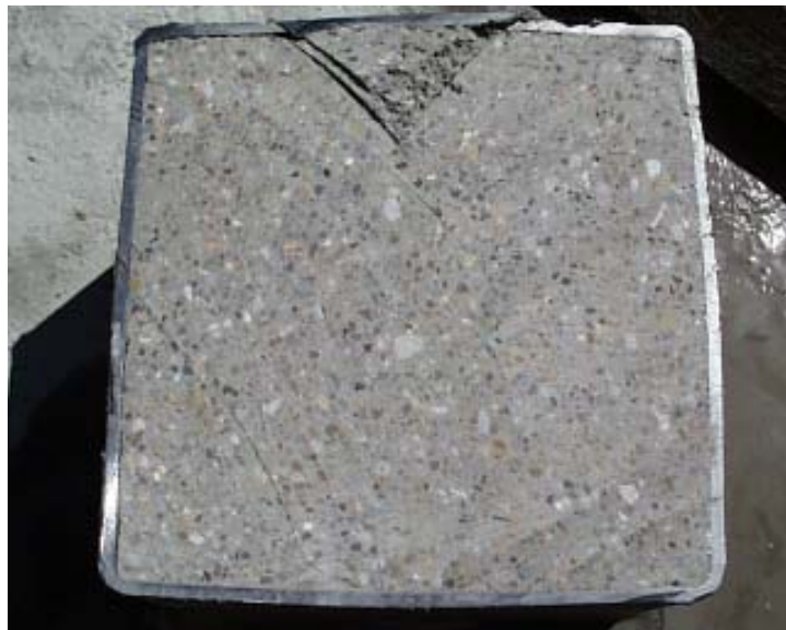
Figure 3-8: Cross-section of Steel Tube with the Grout Mix Design containing 8.5-sack of Cement, Section V
