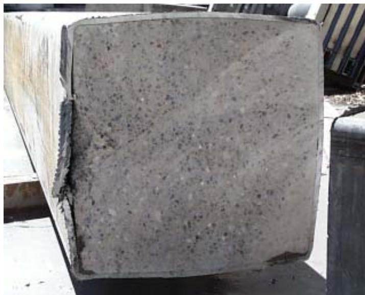
Figure 3-4: Cross-section of Steel Tube with the Grout Mix Design containing 8-sack of Cement, Section IV
