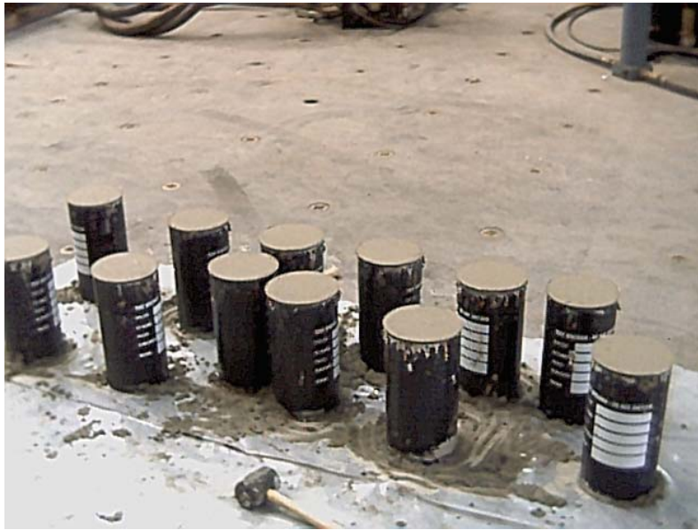
Figure 2-4: 12-in x 6-in Diameter Cylinder Grout Specimens
