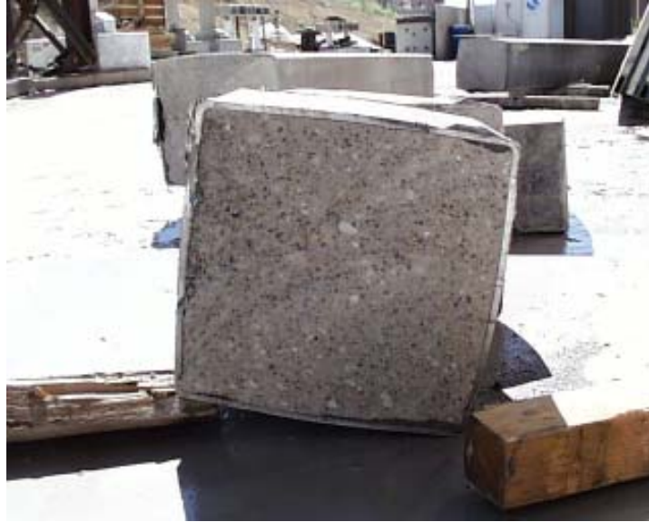
Figure 3-3: Cross-section of Steel Tube with the Grout Mix Design containing 8-sack of Cement, Section III
