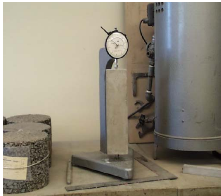
Figure 2-7: Length Comparator with Shrinkage Specimen
