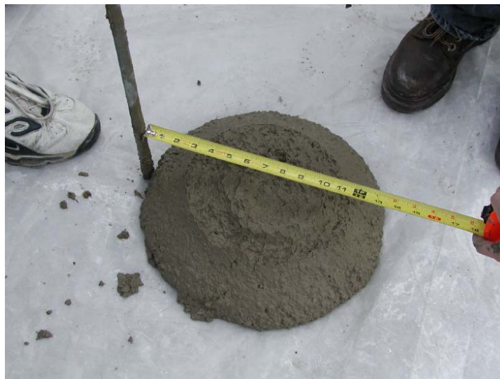
Figure 2-21: Slump Flow Test
