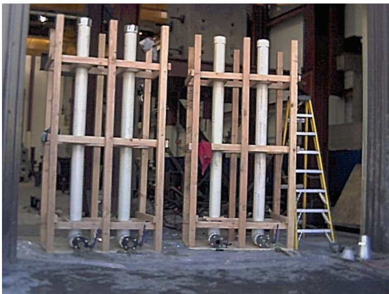
Figure 2-2: 10-ft x 6-in Diameter PVC Pipe Apparatuses
