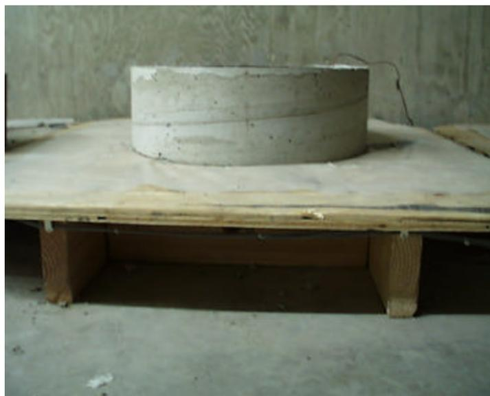
**Figure 4-6. (a) Steel ring with the strain gages and sonotube mold ready for the concrete ring cast; (b) wooden platform supporting the setup for the cracking tendency and hydration tests. Note the thermocouple on the upper right going into the concrete.**
