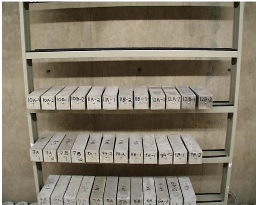
**Figure 4-3. (a) Drying shrinkage specimen molds; (b) Custom built storage shelf for drying shrinkage specimens.**
