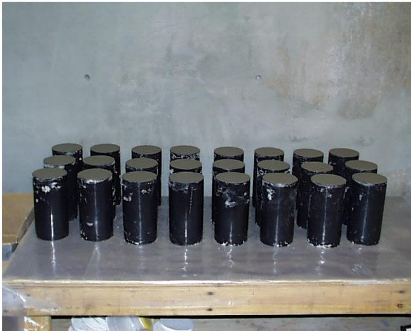
**Figure 4-4. (a) Length comparator reading of a drying shrinkage specimen; (b) 24 cylinders cast for each trial mix design.**
