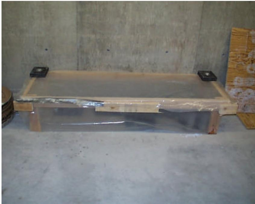
**Figure 4-2. (a) and (b) Overview of the moist box used for the good curing method, in which specimens were moist cured for three days.**
