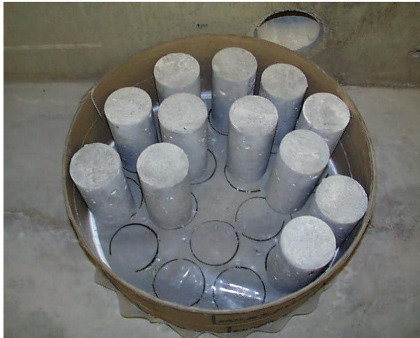
**Figure 4-5. (a) Cylinder test for compressive strength in the concrete lab; (b) Box where all specimens were placed 24 hours after cast to be sprayed with curing compound.**
