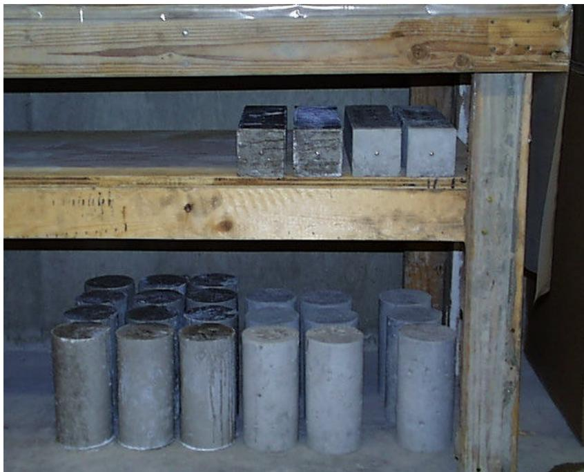
**Figure 4-1. (a) Basement of the structural lab where a table supported the specimens during cast and poor cure; (b) Specimens in poor curing condition.**
