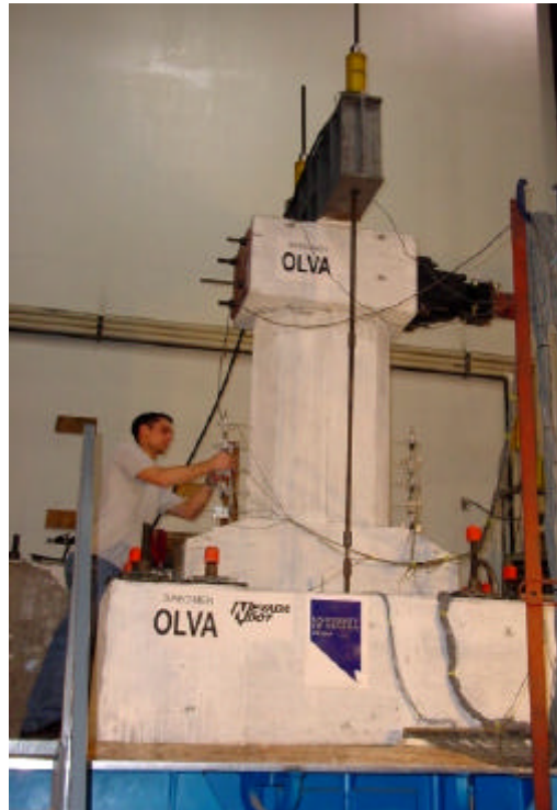
Fig. 2 Nathan Johnson of UNR prepares a model for shake-table testing.
