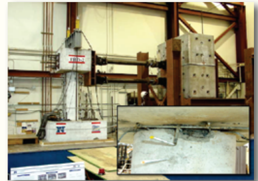
Figure 4 - Shake table test setup and close-up of a hinge after failure
