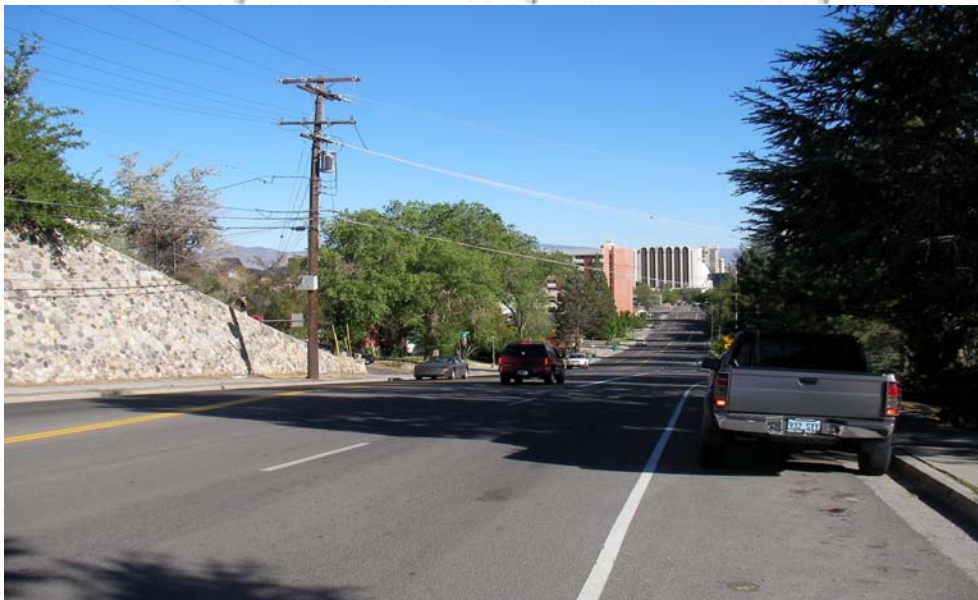
An example of a difficult-to-see marked crosswalk after the hill
