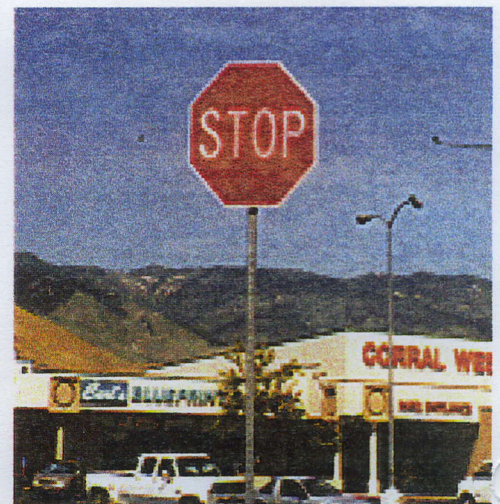
Photo 1, Polycarbonate Stop Sign installed at NDOT west exit.
