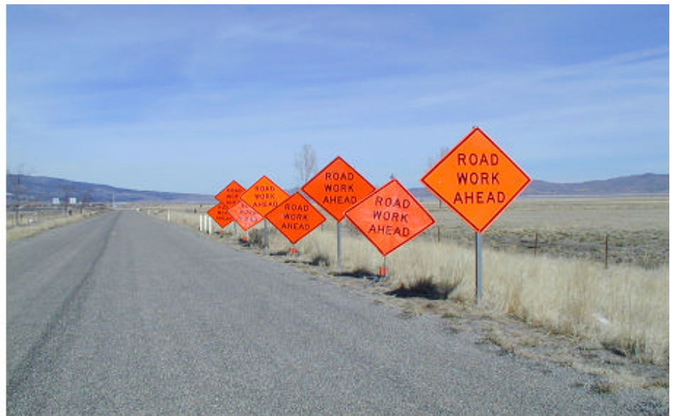
Figure 3. Test section with Endurance Signs.
