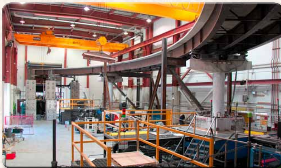
Figure 5: 3-Span Curved Bridge on 4 Shake Tables
