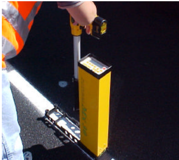
Photo 3. Monitoring of initial retroreflectivity values of the applied pavement marking in accordance with ASTM D4061 testing procedures.
