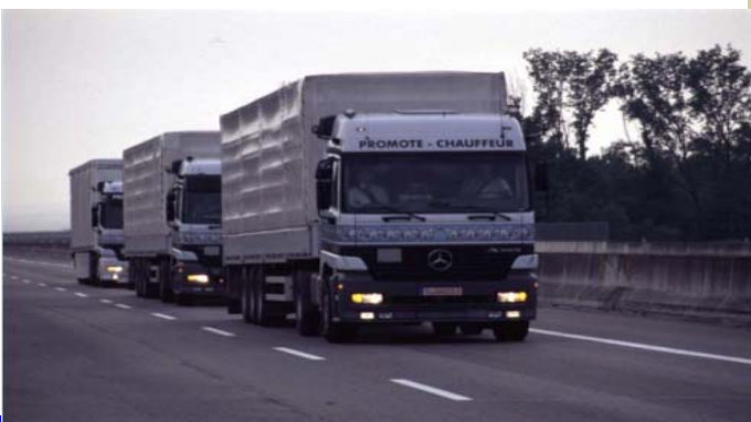
The 3-truck platoon demonstration in the CHAUFFEUR Project by the European Commission (Source: www.itsforum.gr.jp )
