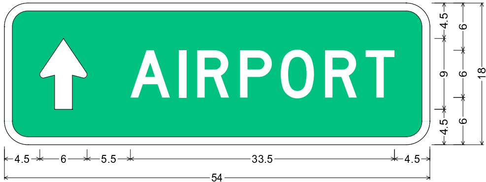
GNV6-1_54x18; 3.0" Radius, 1.0" Border, White on Green; Standard Arrow Custom 9.0" X 6.0" 90°; "AIRPORT" D;
