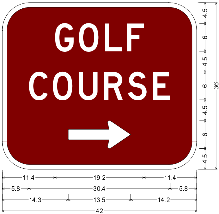
GNV45-2R_42x36; 6.0" Radius, 1.0" Border, White on Brown; "GOLF" D; "COURSE" D; Standard Arrow Custom 13.5" X 6.0" 0°;
