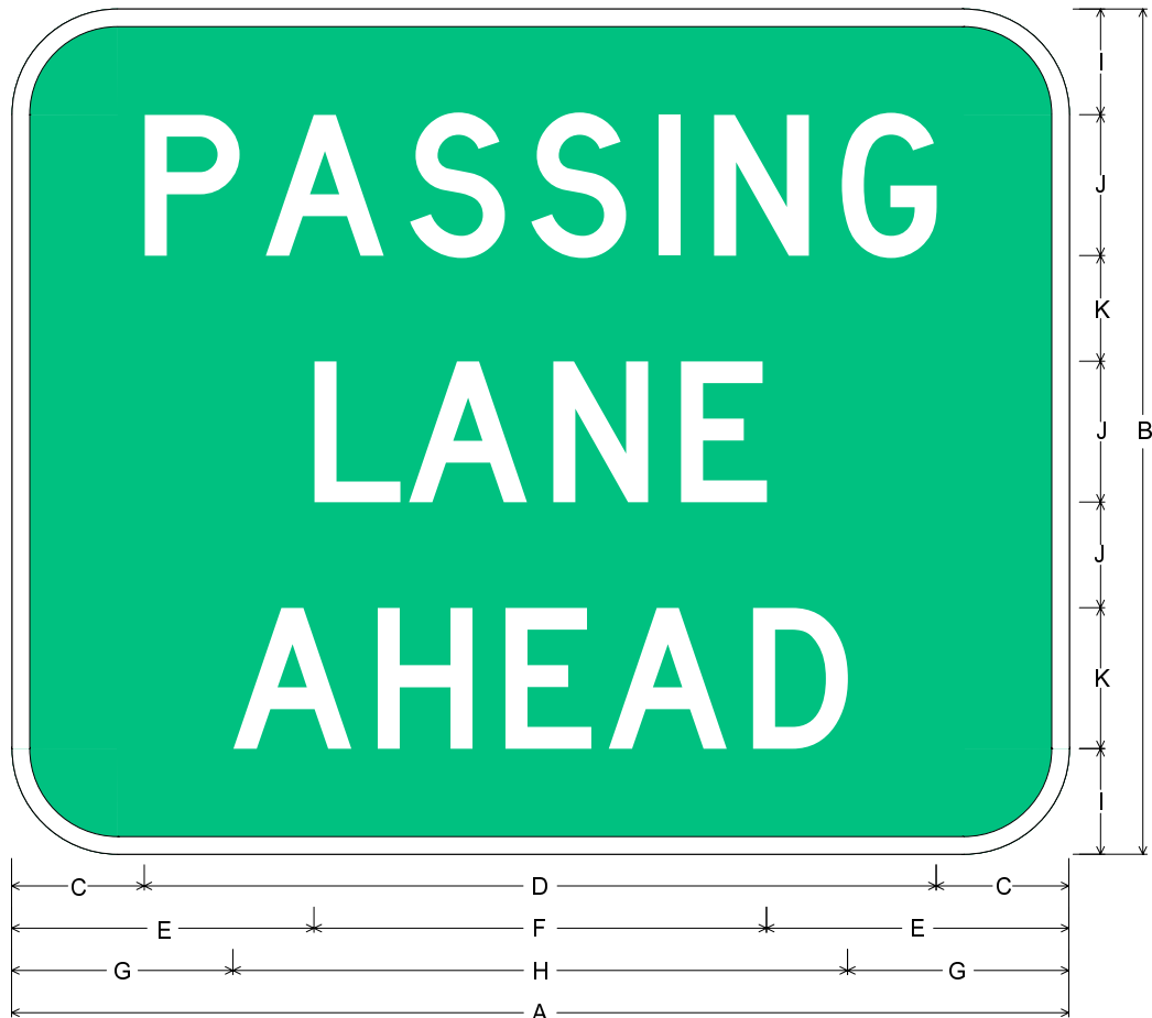
GNV5-1_60x48; 6" Radius, 1" Border, White on Green; [PASSING] D; [LANE] D; [AHEAD] D;
