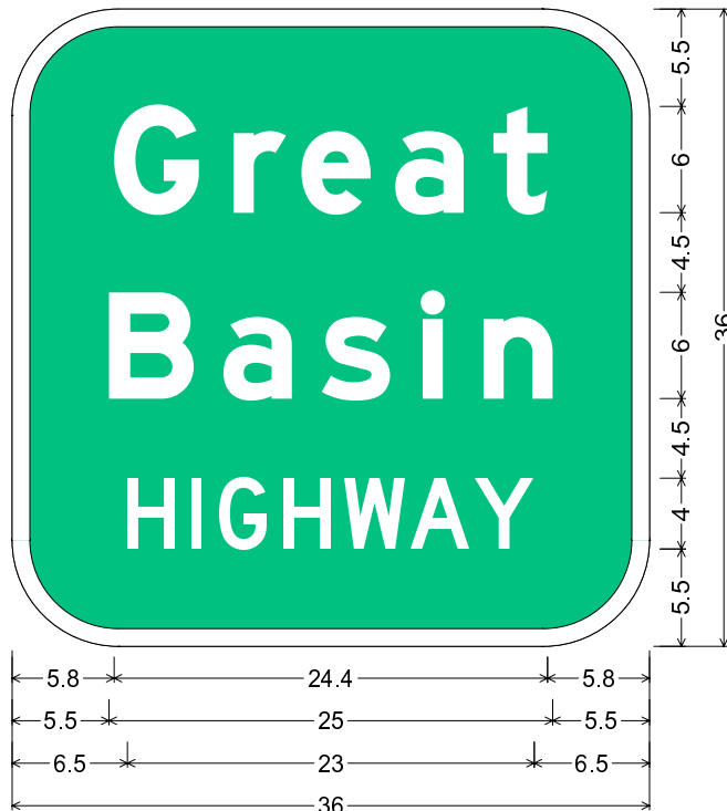
GNV26-3_36x36; 6.0" Radius, 1.0" Border, White on Green; "Great" E Mod; "Basin" E Mod; "HIGHWAY" D;
