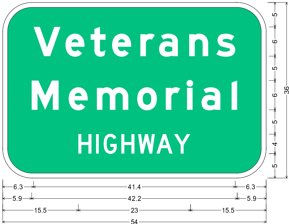
GNV26-1_54x36; 6.0" Radius, 1.0" Border, White on Green; "Veterans" E Mod; "Memorial" E Mod; "HIGHWAY" D;
