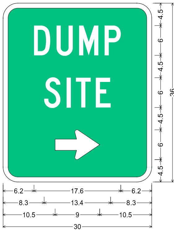
GNV10-2R_30x36; 3.0" Radius, 1.0" Border, White on Green; "DUMP" C; "SITE" C; Standard Arrow Custom 9.0" X 6.0" 0°;
