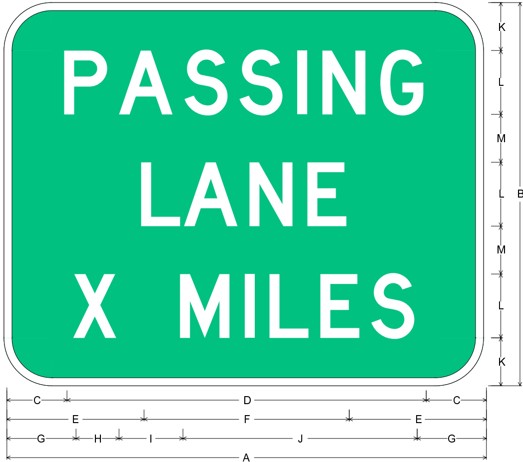
GNV5-2; 6" Radius, 1" Border, White on Green; [PASSING] D; [LANE] D; [X MILES] D;
