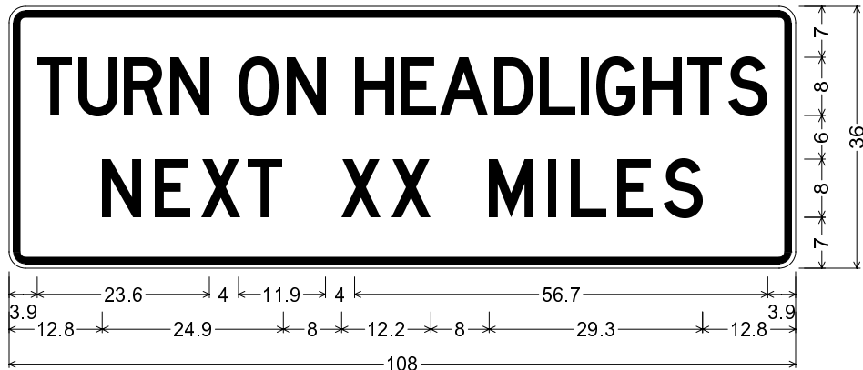
RNV8-3_108x36; 2.3" Radius, 0.9" Border, 0.6" Indent, Black on White; "TURN ON HEADLIGHTS" D 50% spacing; "NEXT XX MILES" D;
