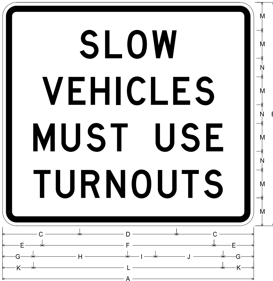
RNV6-1, Black on White; [SLOW] D; [VEHICLES] D; [MUST USE] D; [TURNOUTS] D;
