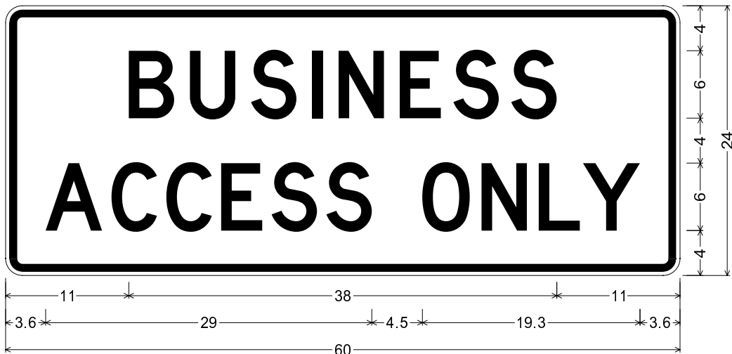
RNV29-1_60x24; 1.5" Radius, 0.6" Border, 0.4" Indent, Black on White; "BUSINESS" D; "ACCESS ONLY" D 75% spacing;
