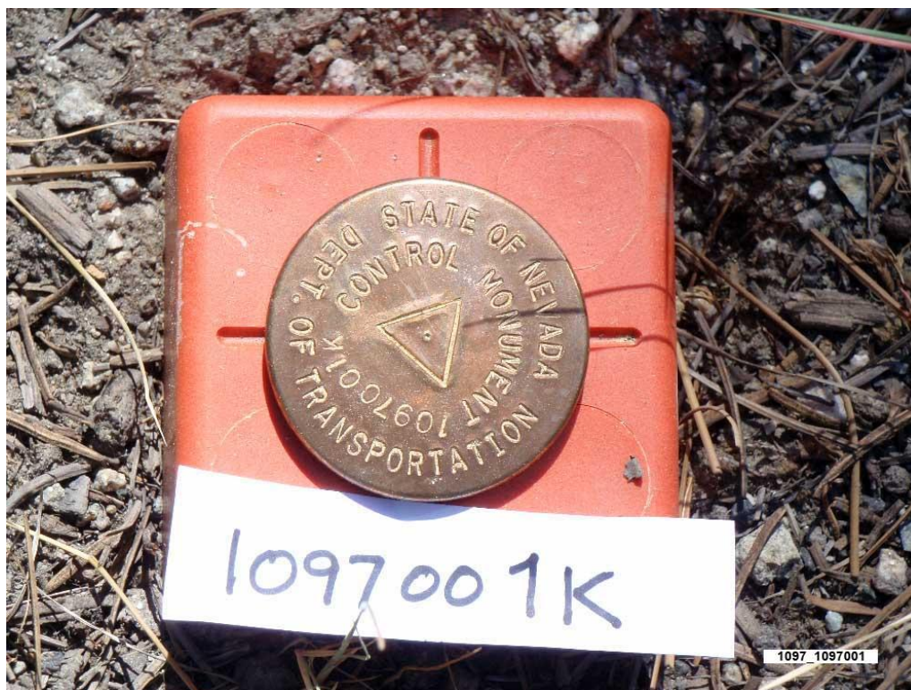
K-Construction Control Point / No Spirit Level Elevations
