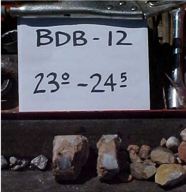
Photo 2. Caliche Sample from Borehole BDB-12
