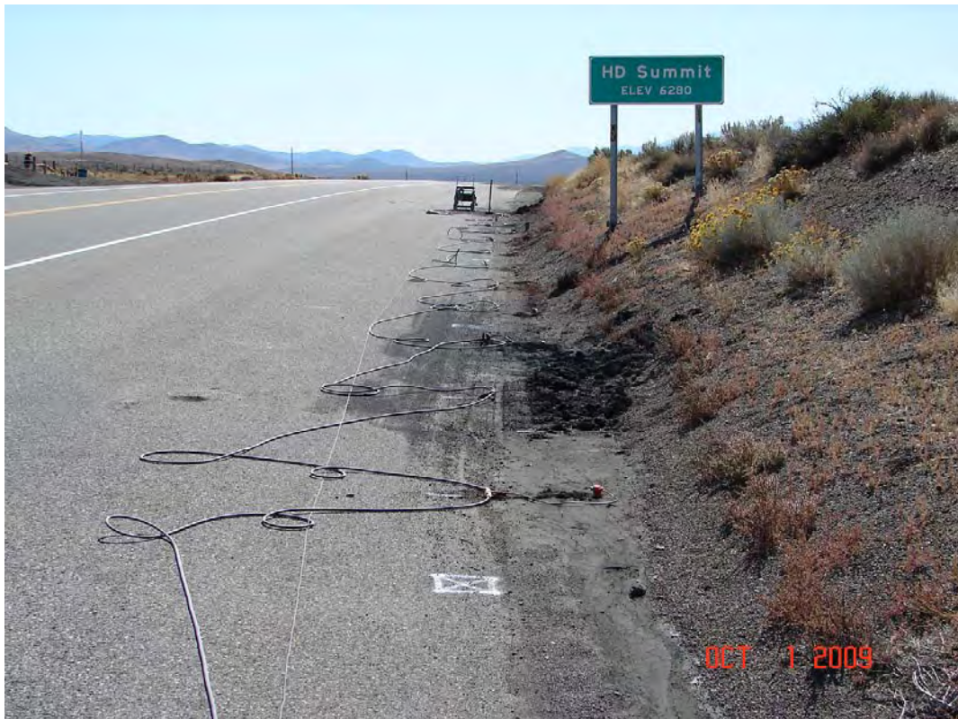
Photo 3. Seismic Refraction Run on West Side of US 93 at HD Summit.
